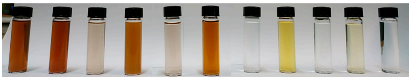
Figure 11. Photo of the extracted samples; from left to the right: I-ethanol, II-ethanol, UF feed, UF retentate, UF permeate, NF600 retentate, NF600 permeate, NF300 retentate, NF300 permeate, RO retentate, RO permeate.
