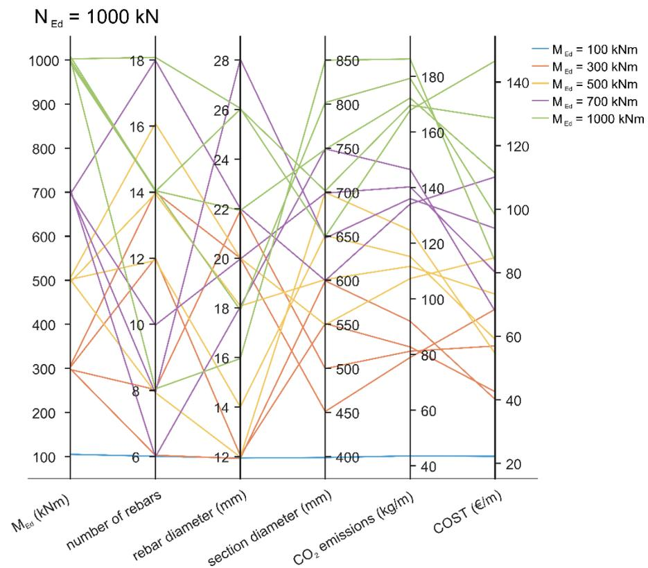
Figure 8. Parallel coordinate representation of the optimum design variables of a reinforced concrete circular cross section loaded with an axial load of 1000 kN for different applied bending moments.
