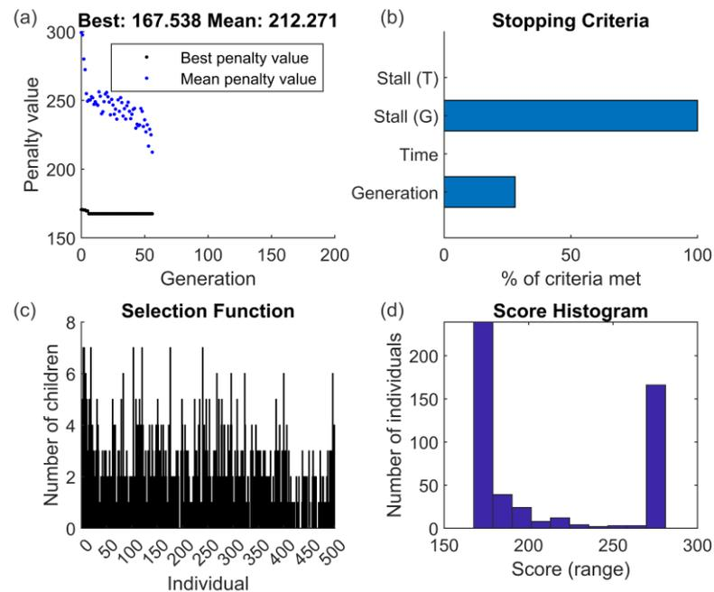
**Figure 4.** Performance of the genetic algorithm (objective function: CO<sub>2</sub> emissions,  $N_{Ed} = 1000$  kN and  $M_{Ed} = 1000$  kNm): (a) progress of the genetic algorithm; (b) stopping criteria; (c) population size; (d) score histogram.
