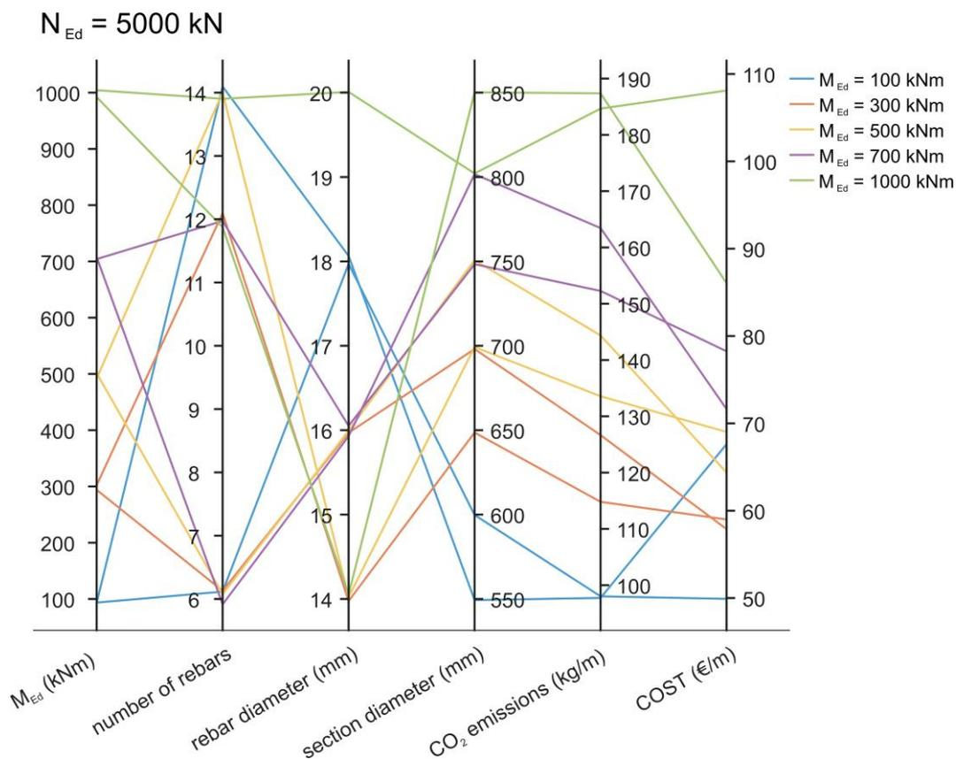
**Figure 10.** Parallel coordinate representation of the optimum design variables of a reinforced concrete circular cross-section loaded with an axial load of 5000 kN for different applied bending moments.
