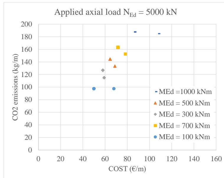
**Figure 7.** Pareto front for a reinforced concrete circular cross section loaded with an axial load of 5000 kN for different applied bending moments.
