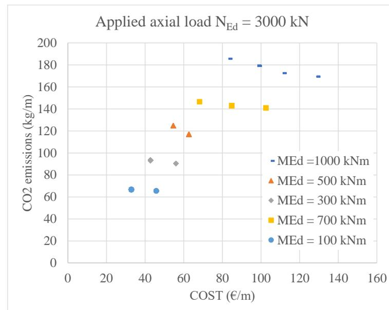
**Figure 6.** Pareto front for a reinforced concrete circular cross section loaded with an axial load of 3000 kN for different applied bending moments.
