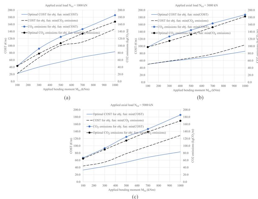
Figure 3. Optimal material costs and optimal CO<sub>2</sub> emissions for different applied bending moments (a) at an applied axial load of 1000 kN, (b) at an applied axial load of 3000 kN, and (c) at an applied axial load of 5000 kN.
