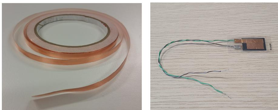
**Figure 4.** Left: copper adhesive tape. Mosborne01, CC BY-SA 3.0 <https://creativecommons.org/licenses/by-sa/3.0>, accessed on 5 June 2023, via Wikimedia Commons. Right: prototype of PZ harvester based on PHBV, where the copper layer can be seen. Development and photograph by Luna Geber Engineering, reproduced with permission.
