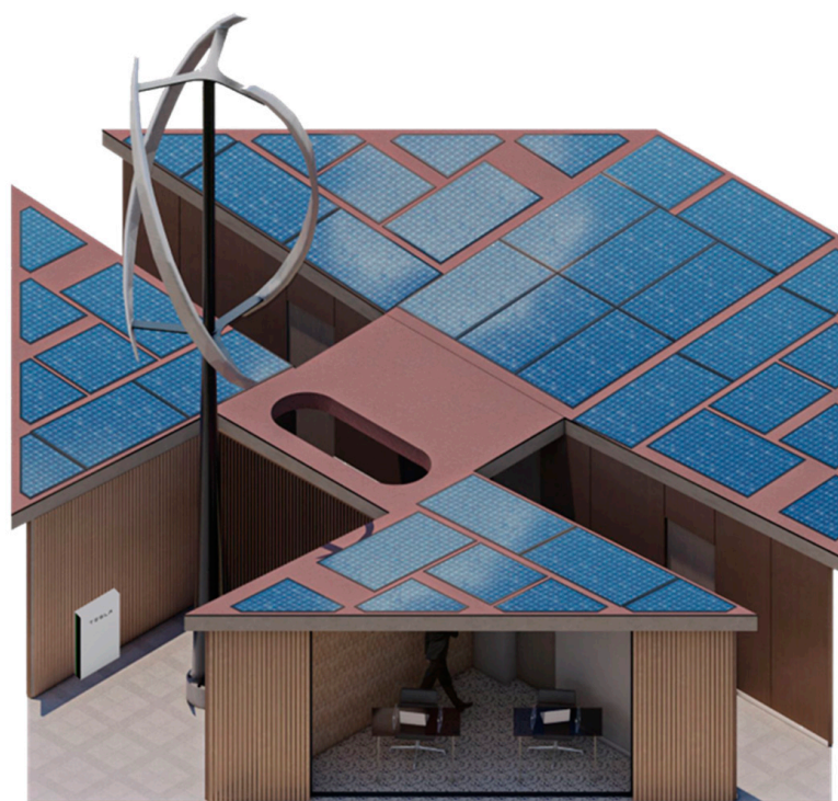
Figure A4. Architectural model of building configuration C, including the PV panels, wind turbine, and electric storages.
