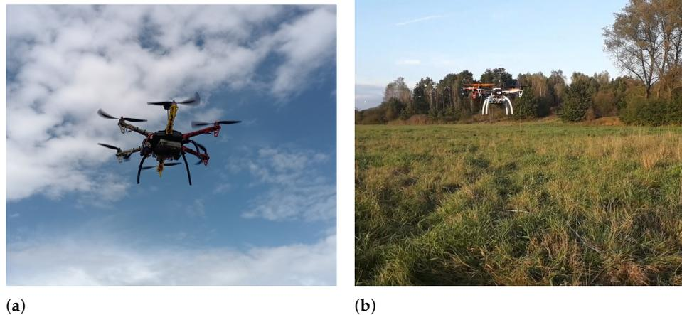
**Figure 8.** Drones during the field tests. (a) hexacopter in the air while navigating to the next point; (b) quadcopter during the take-off.
