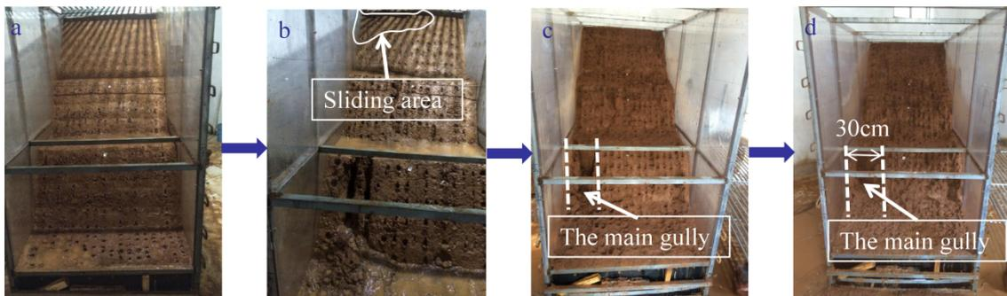
**Figure 8.** Scour failure process during three rounds of rainfall: (a) First round of the first rainfall event lasted for 5 min, (b) First round of the first rainfall event lasted for 70 min, (c) First round of the second rainfall event lasted for 120 min, (d) Third round of the third rainfall event lasted for 120 min.
