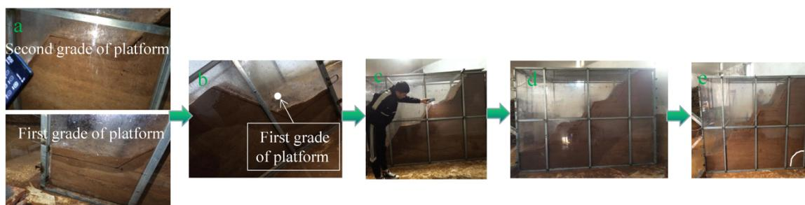
**Figure 10.** Rainwater infiltration process within the slope model: (a) After 30 min of the first round of the first rainfall event, (b) After 120 min of the first round of the first rainfall event, (c) 5.2 h after the first round of the second rainfall event, (d) After 120 min of the second round of the third rainfall event, (e) After 120 min of the third round of the first rainfall event.
