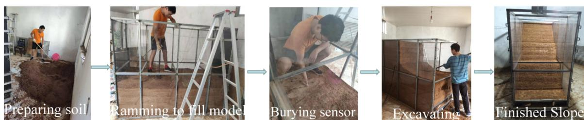
Figure 5. Slope model construction process.
