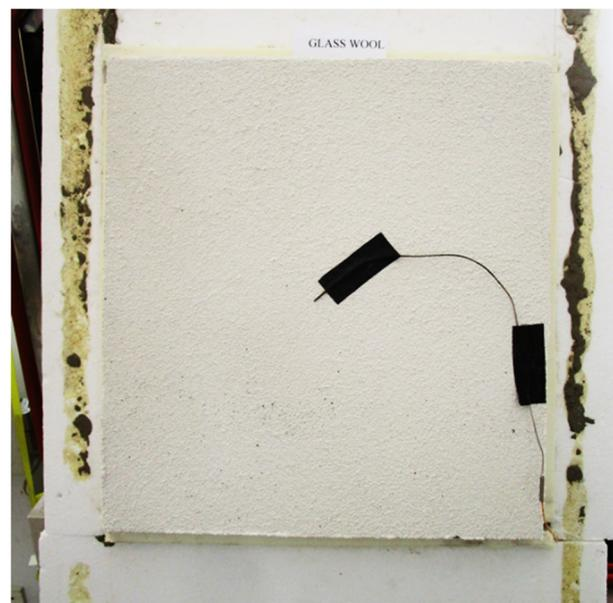
**Figure 4.** Temperature sensor position on the ETICS surface.
