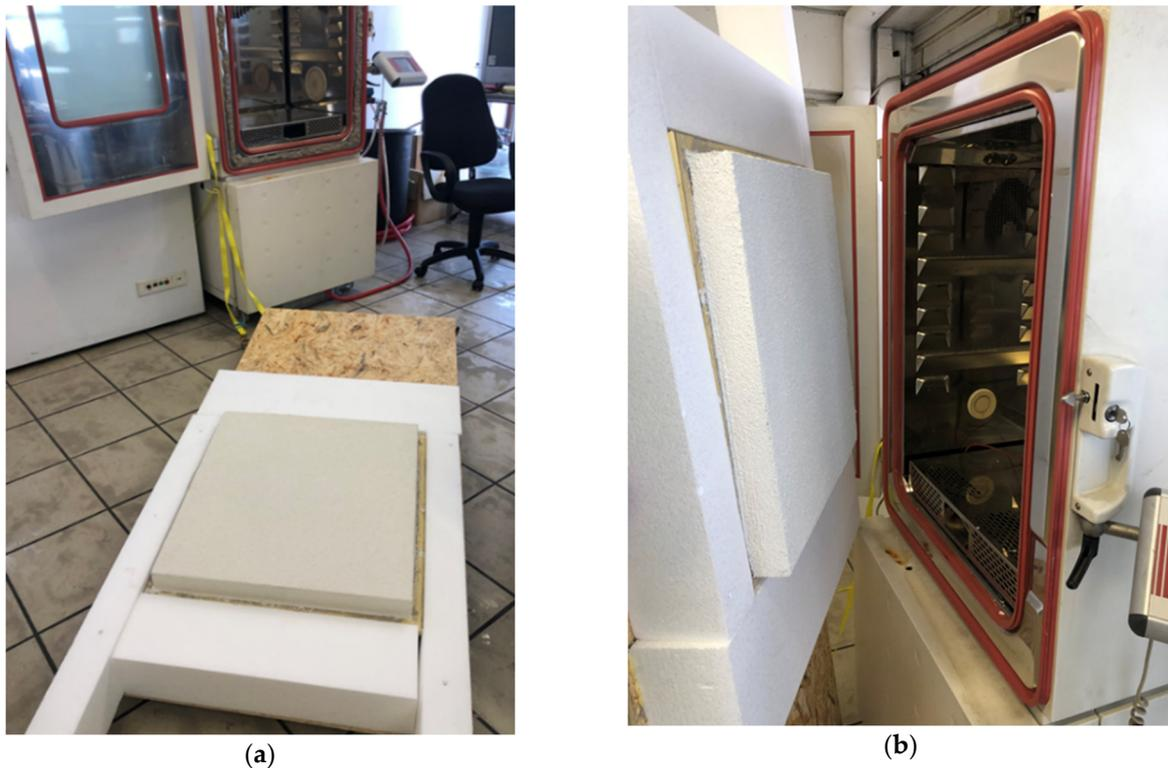
**Figure 3.** Placement of the sample inside the climatic chamber: (a) sample outside the chamber, placed on a stand; (b) sample being placed as the door of the climatic chamber, before addition of temperature sensors.
