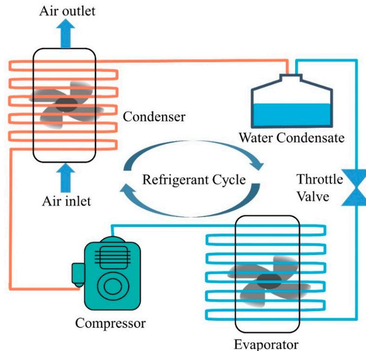
**Figure 4.** Diagram of refrigerant evaporation–condensation cycle.
