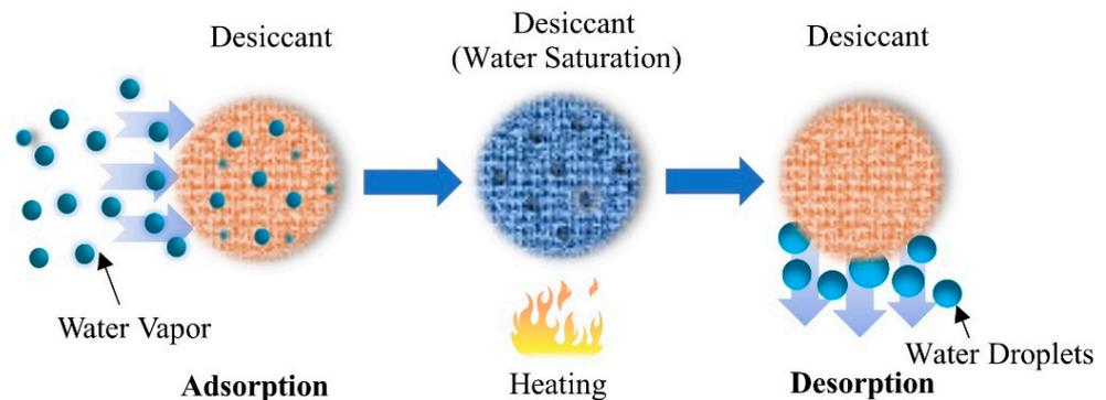
**Figure 5.** Diagram of the desiccant-based atmospheric water harvesting.
