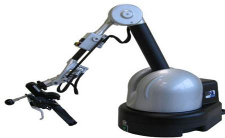
**Figure 4.** Haptic feedback device Virtuose 6D TAO.
