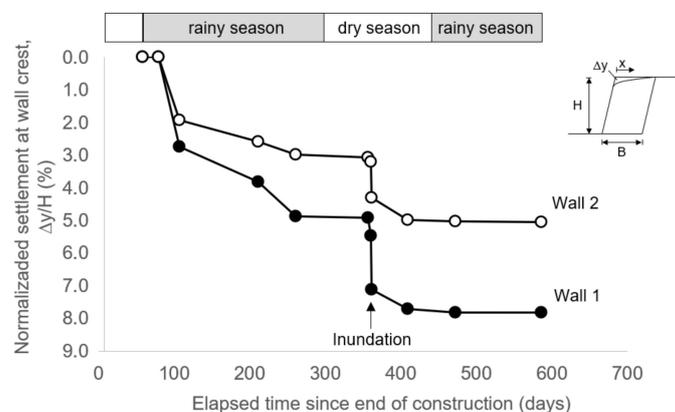
**Figure 11.** Vertical displacements at the wall top ( $x/B = 0.24$ ).
