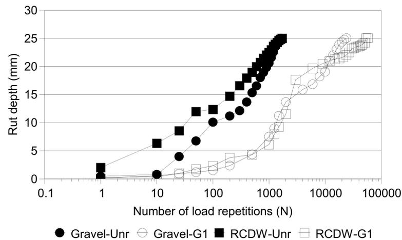
Figure 4. Rut displacement versus number of load repetitions.
