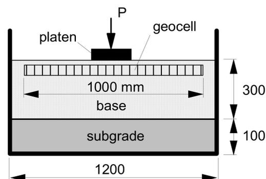
Figure 5. Tests on unpaved roads reinforced with geocells [62], modified.
