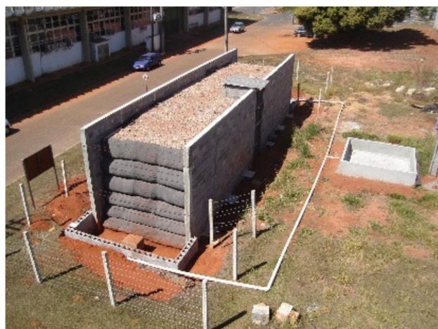
**Figure 9.** Complete view of the test facility showing the water reservoirs and main reservoir [55].
