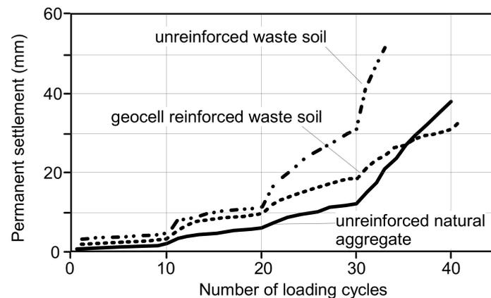
Figure 6. Settlement versus number of loading cycles [62], modified.
