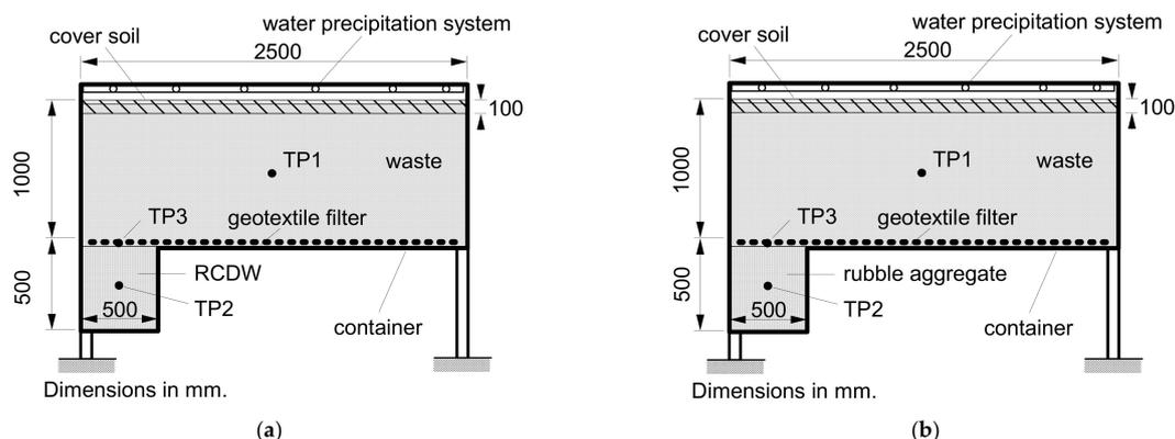
Figure 12. Waste containers: (a) container C1; (b) container C2 [77].
