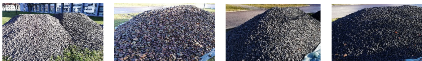
Figure 1. Tested SBM as fill material from left to right: recycled concrete (RC), track ballast (TB), blast furnace slag (BFS), electric furnace slag (EFS). Source: Schneider.
