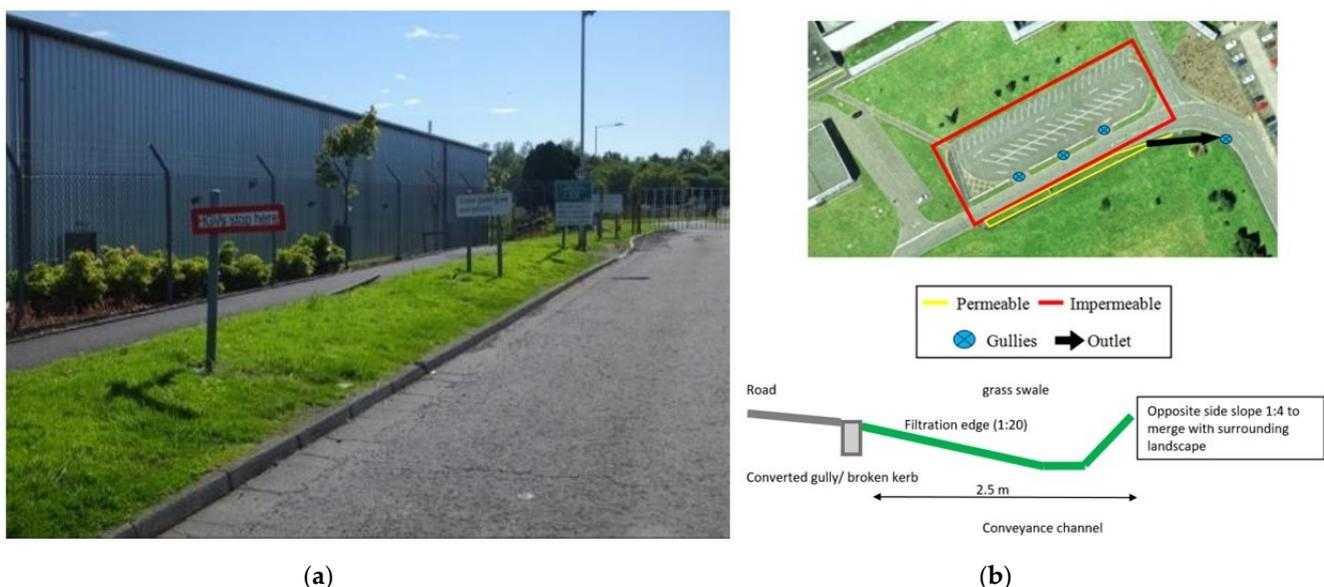
**Figure 15.** (a) Grass verge at Company B approach road, which could be converted to be a swale. (b) Technical schematic for the retrofit swale.
