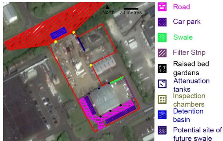
**Figure 8.** Layout of proposed SUDS features at the Company A site (Google DigitalGlobe, 2016). Inspection chambers shown in yellow on image for clarity. The area indicated with red hatching covers the additional catchment from the adjacent public road.
