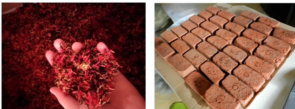
**Figure 2.** MAST (Mattone in Argilla con Scarti Tessili—Clay Brick from Textile Waste): from textile waste to experimental specimens. On the left, shredded polyester threads; on the right, clay bricks obtained with different percentages of polyester waste.
