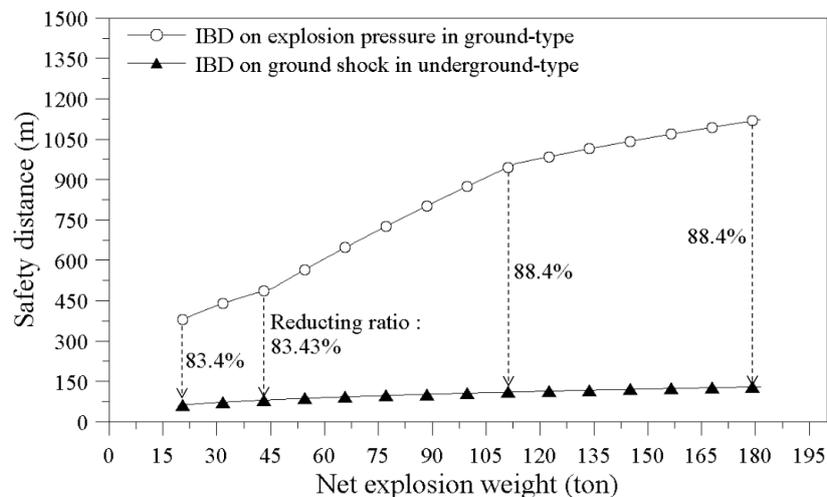
Figure 3. Comparison of dominant safety distances between ground-type and underground-type ammunition magazines (which are IBD for explosion pressure and IBD for ground shock, respectively).
