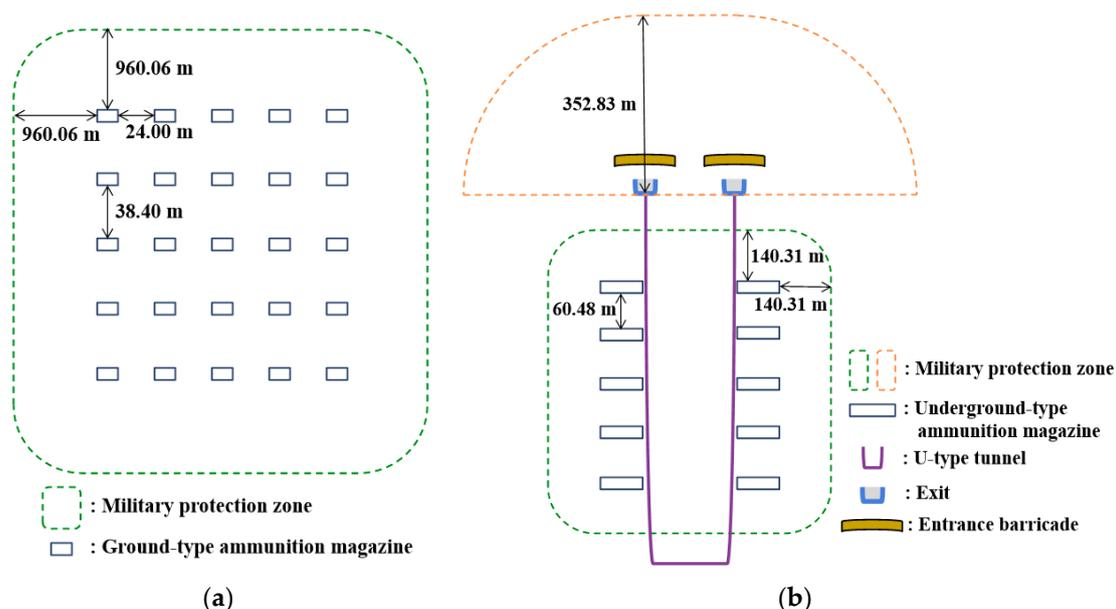
**Figure 5.** Military protection zones estimated in example. (a) Ground-type ammunition facility; (b) Underground-type ammunition facility.
