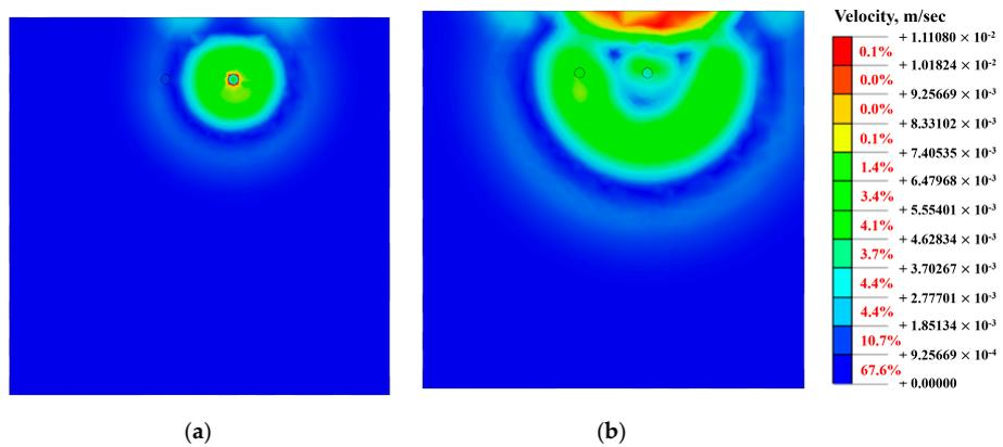
Figure 11. Results of numerical simulation for velocity of ground particle in Case 3: (a)  $t = 1.5 \times 10^{-2}$ ; (b)  $t = 3.0 \times 10^{-2}$ .
