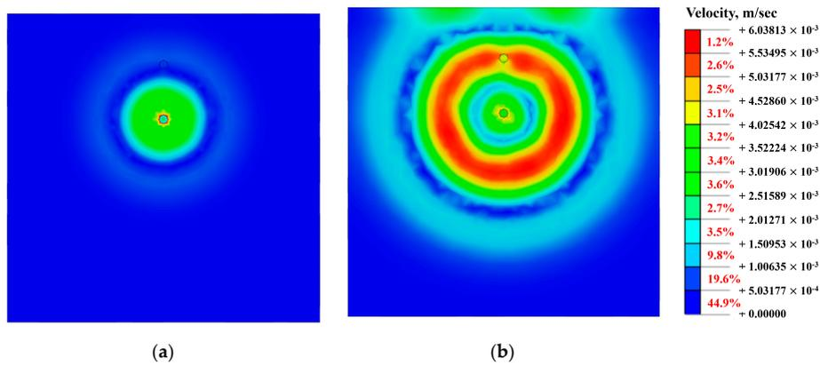
Figure 10. Results of numerical simulation for velocity of ground particle in Case 2: (a)  $t = 1.5 \times 10^{-2}$ ; (b)  $t = 3.0 \times 10^{-2}$ .
