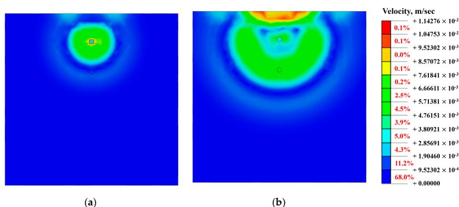
**Figure 9.** Results of numerical simulation for velocity of ground particle in Case 1: (a)  $t = 1.5 \times 10^{-2}$ ; (b)  $t = 3.0 \times 10^{-2}$ .
