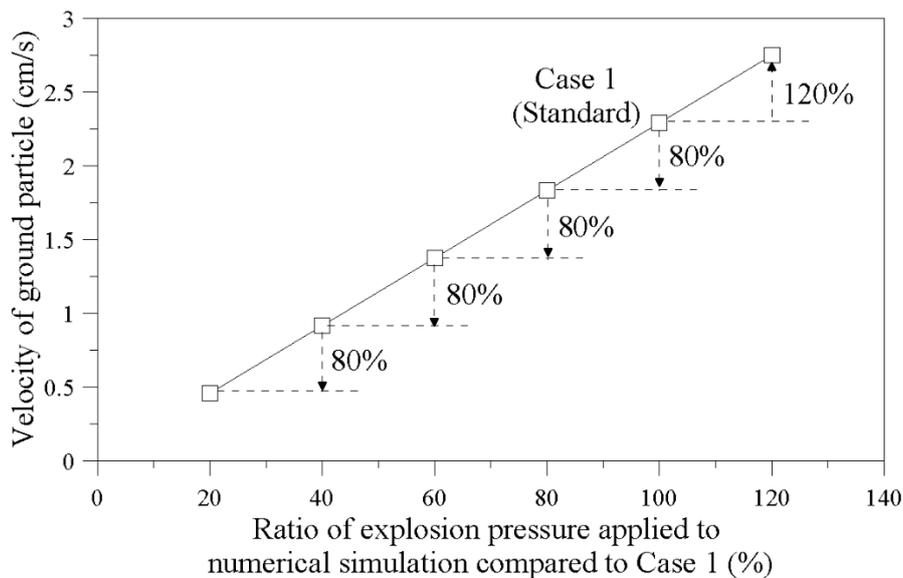
Figure 12. Reduction degree of ground particle velocity in accordance with decrease in explosion pressure applied at chamber wall.
