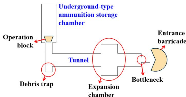
**Figure 6.** Schematic diagram of protective structures in an underground-type ammunition magazine.
