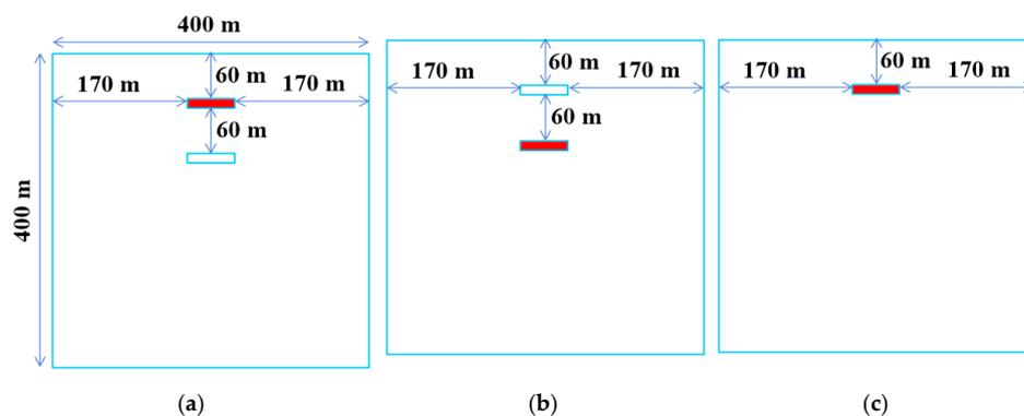
**Figure 8.** y-z coordinate of each simulation case for estimating ground shock effect to one chamber in explosion of another chamber: (a) effect of ground shock to adjacent downward chamber (Case 1); (b) effect of ground shock to adjacent upward chamber (Case 2); (c) effect of ground shock to adjacent chamber at same depth (Case 3).
