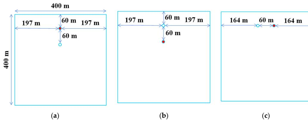
**Figure 7.** x-z coordinate of each simulation case for estimating ground shock effect to one chamber in explosion of another chamber: (a) effect of ground shock to adjacent downward chamber (Case 1); (b) effect of ground shock to adjacent upward chamber (Case 2); (c) effect of ground shock to adjacent chamber at same depth (Case 3).
