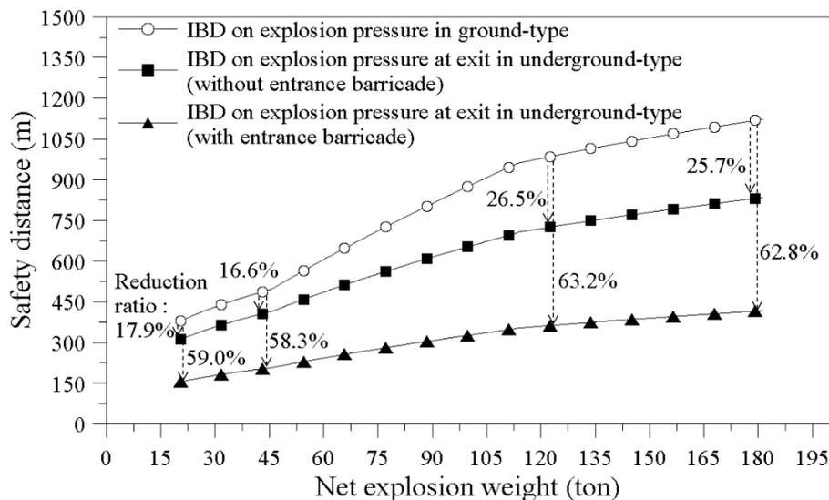
**Figure 4.** Comparison of dominant safety distances between ground-type and underground-type ammunition magazines (which are IBD for explosion pressure and IBD for explosion pressure at exit, respectively; considering the entrance with and without barricade).
