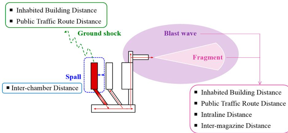
Figure 2. Schematic diagram of safety distances for an underground-type ammunition magazine.
