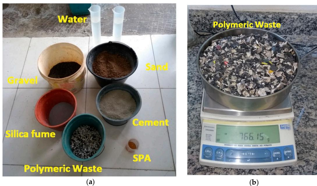
**Figure 2.** Agglomerate materials: cement and silica; natural aggregates: sand and gravel; artificial aggregates: polymeric waste and water. (a) All materials used in the mixtures and (b) weighing of the polymeric waste for concrete mixing.
