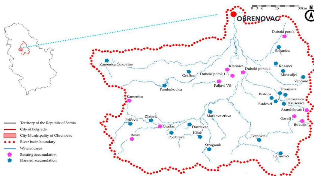
**Figure 6.** GIS visualization showing existing (magenta) and planned (blue) accumulations in the Kolubara river basin. Source: According to “SRBIJAVODE” Water Authority [25].
