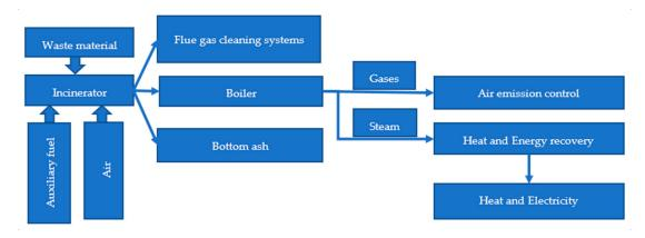
Figure 1. Process of incineration of municipal solid waste management.
