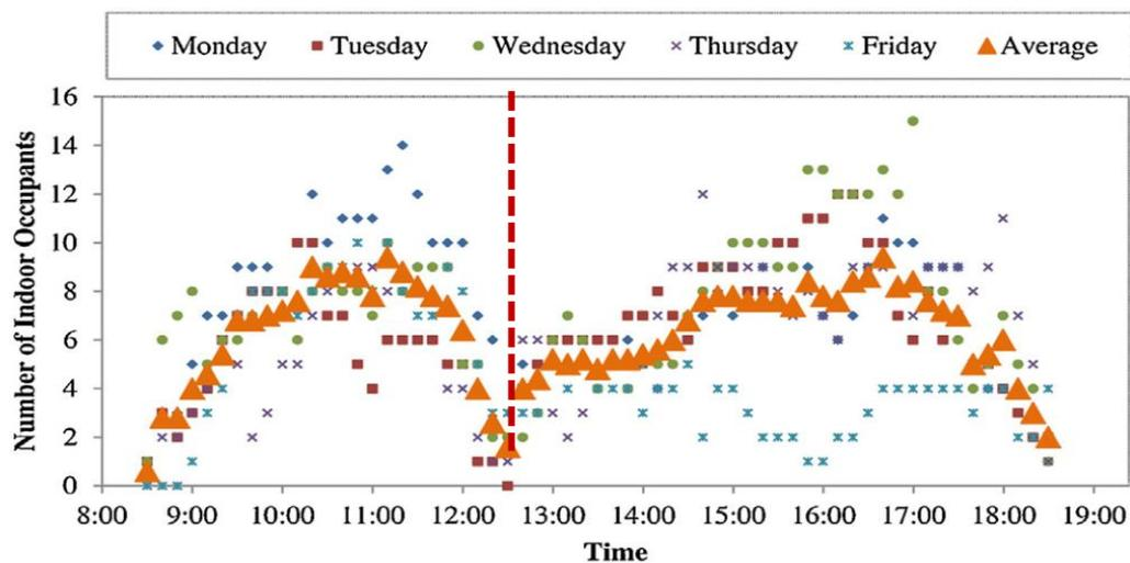
Figure 4. Time-varying indoor occupant number of a multiple-occupant office.
