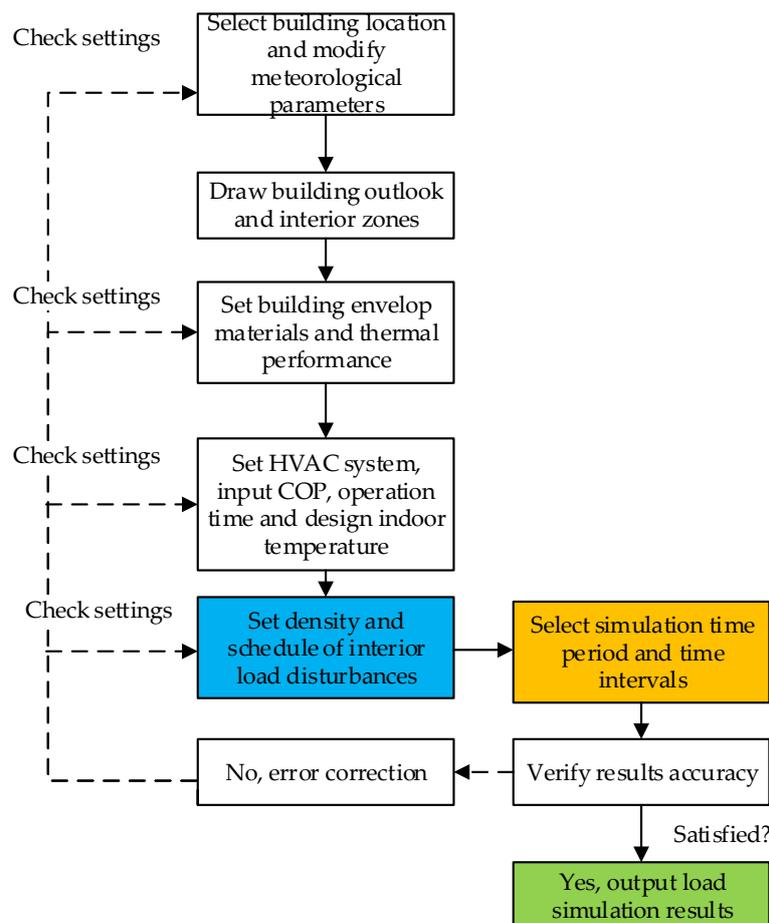
**Figure 2.** Flow chat of building load simulation based on DesignBuilder tool.
