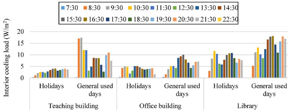
Figure 15. Interior cooling load calculation results of case buildings.
