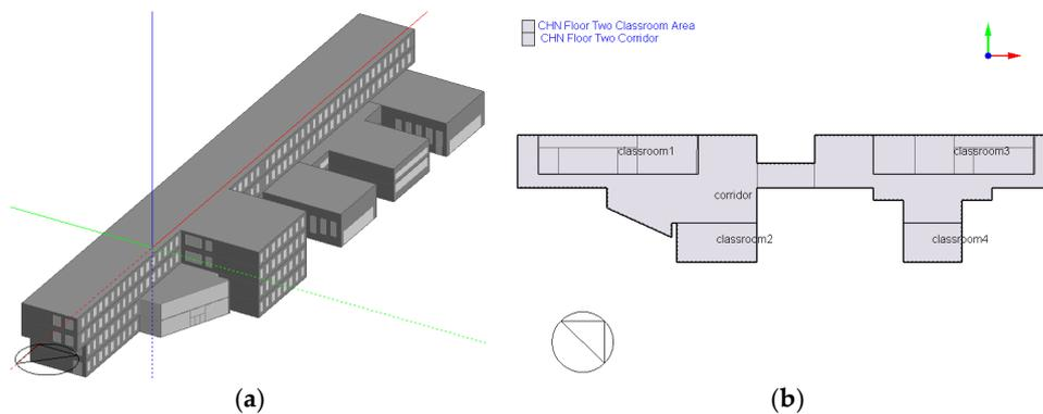
Figure 16. Building cooling load simulation model based on DesignBuilder of the teaching building. (a) External view and (b) interior division of standard floor.
