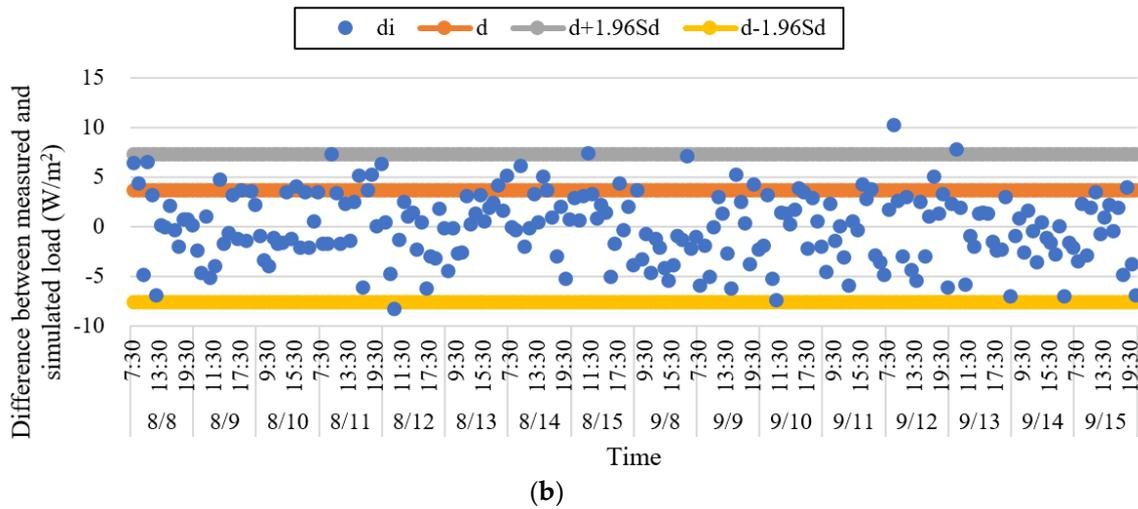
**Figure 20.** Comparison of simulated and actual building cooling loads of the office building. (a) Time-varying loads and (b) consistency validation.
