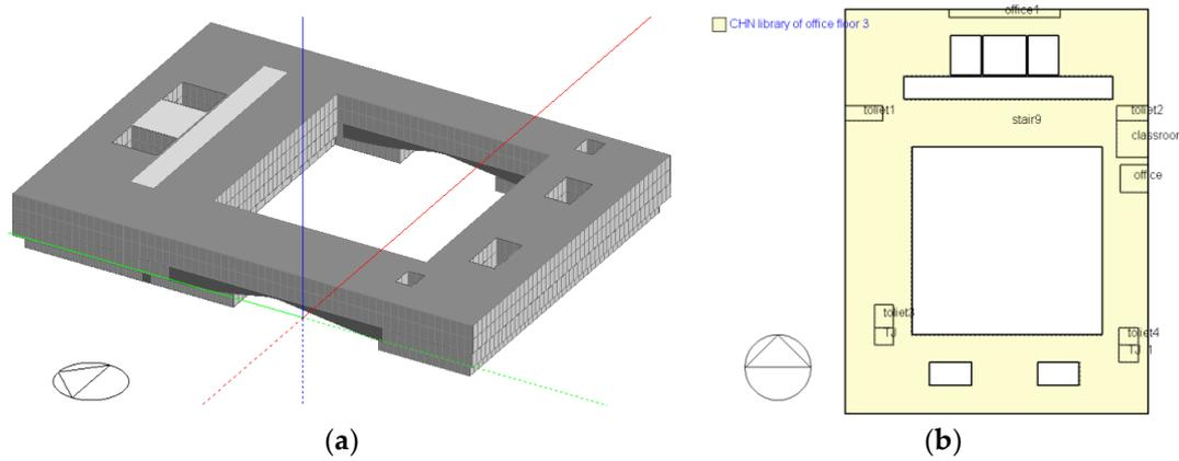
**Figure 18.** Building cooling load simulation model based on DesignBuilder of the library. (a) External view and (b) interior division of standard floor.
