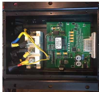
Figure 19. Electronic control unit of DAL-ECR.
