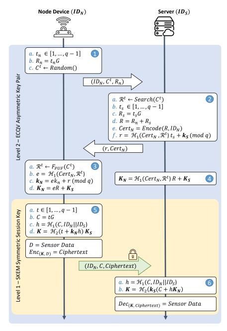
**Figure 2.** 2-level security key establishment protocol. The computations are grouped into six steps, each indicating sequential operations at the sender and receiver.
