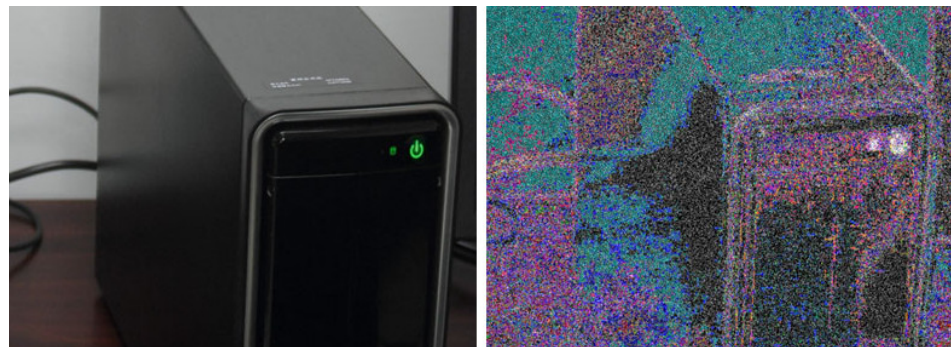
Figure 2. Example of ELA. (Left), image with power button manipulated. (Right) Resulting image after ELA, usually mostly black, except for the two manipulated areas that have differences in compression.
