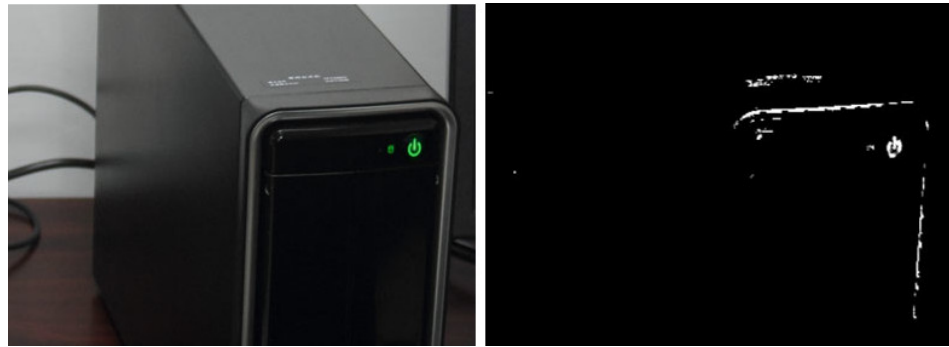
Figure 3. Example of DWT method. (Left), image power button manipulated. (Right) Results of the DWT (variations are enhanced).
