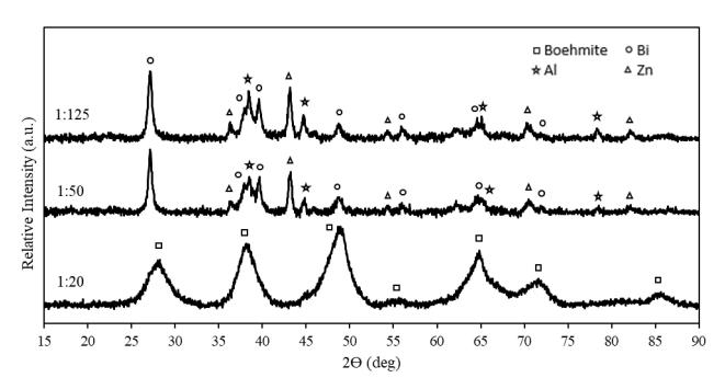
Figure 8. Hydrolysis residues of ternary composite Al-5% Bi-5% Zn at various mass ratios.
