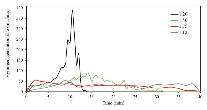
Figure 7. Hydrogen generation rates of Al-5% Bi-5% Zn composite hydrolyzed at various mass ratios.
