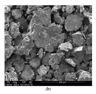
**Figure 1.** Secondary electron SEM micrographs of as-received Al (a) and mechanochemically processed Al-5% Bi-5% Zn composite (b) particles.
