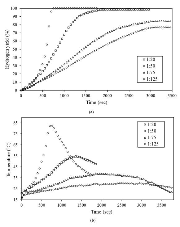
**Figure 6.** Effect of mass ratio on hydrogen yield of Al-5% Bi-5% Zn (a) and the change in reaction temperature during hydrolysis (b).
