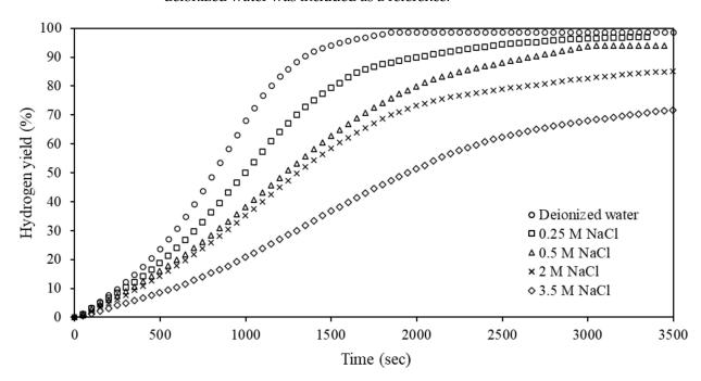
**Figure 10.** Hydrogen yield of Al-5% Bi-5% Zn composite reacting with different concentrations of NaCl solutions at room temperature.
