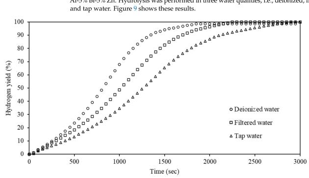
Figure 9. Hydrogen yield curves of Al-5% Bi-5% Zn hydrolyzed using different water qualities.
