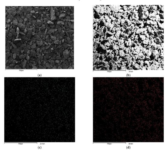
**Figure 3.** Secondary SEM micrograph of the surface of Al-5% Bi-5% Zn (**a**) and the corresponding EDS mappings for Al (**b**), Bi (**c**), Zn (**d**).
