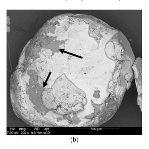
**Figure 2.** Backscattered electron SEM micrographs of mechanochemically processed Al-2.5% Bi-7.5% Zn (a) and Al-2.5% Bi-2.5% Zn composite (b) to emphasize the incomplete composite constituency distribution (indicated by arrows).
