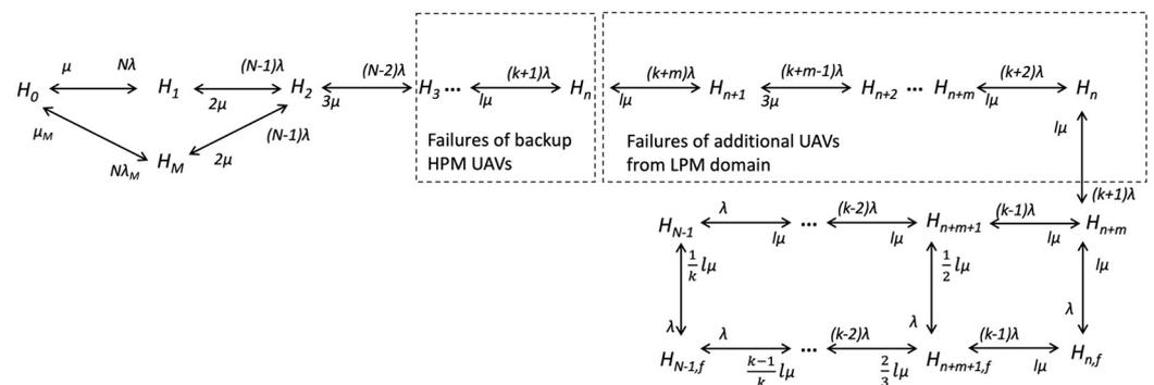
Figure 5. State transition graph for HPM with possibility of using UAVs from LPM cluster.
