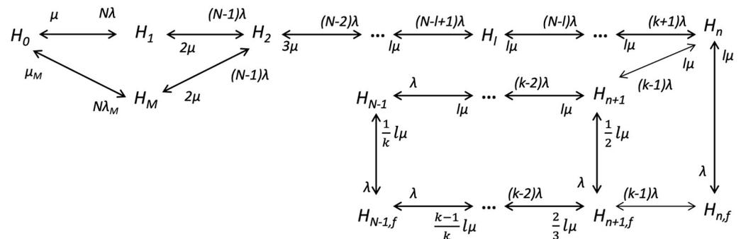
**Figure 2.** State transition graph of a Markov chain for HPM cluster with maintenance of batteries in autonomous mode.
