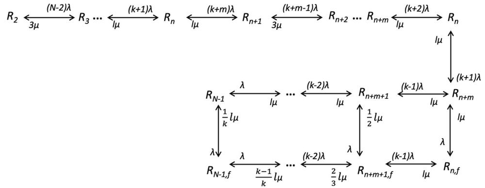
Figure 7. Markov chain for subsystem R.
