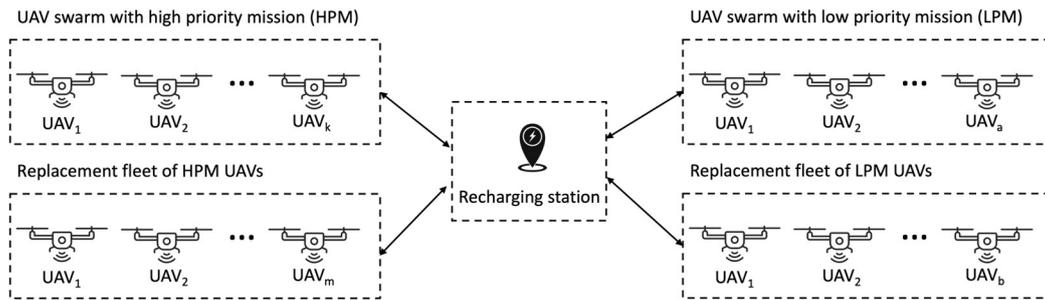
**Figure 1.** Framework for UAV swarm operations during special missions.
