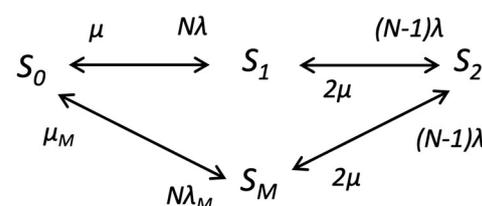
Figure 6. Markov chain for subsystem  $S$ .
