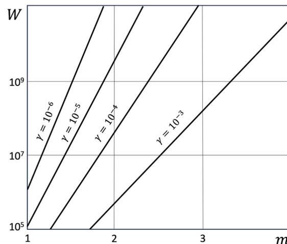
**Figure 9.** Dependability enhancement factor as a function of the number of extra redundant UAVs from the LHM sector.
