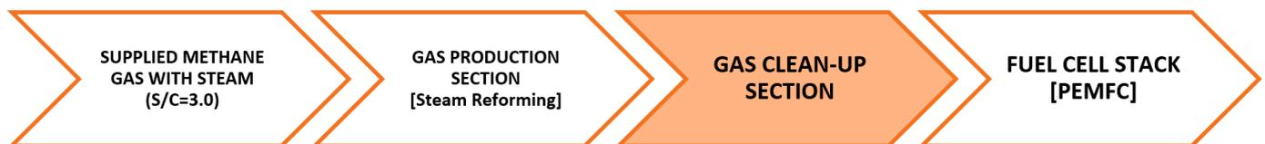
Figure 1. Schematic of methane reforming PEMFC system.
