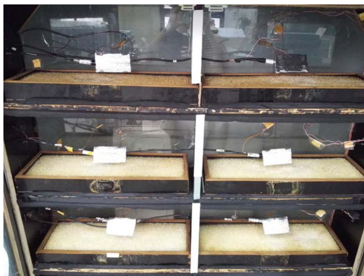
Figure 4. Image of the desiccant modules embedded in the window.
