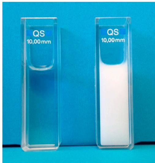
**Figure 3.** Photograph of aqueous 3 wt. % HPC sample below switching temperature (left), above switching temperature (right).
