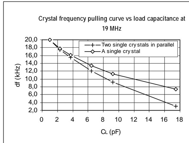
**Figure 8.** A comparison of pullability exhibited by a single- and dual-crystal unit operated in series with load capacitance at the frequency of 19 MHz.
