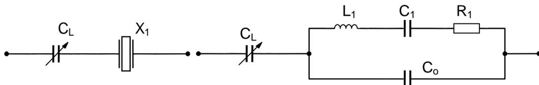
**Figure 2.** Quartz crystal unit operated with a load capacitance.
