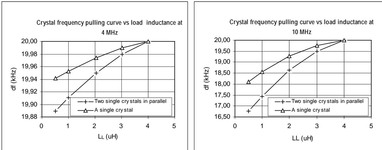
**Figure 9.** A comparison of pullability exhibited by a single- and dual-crystal unit operated in series with load inductance at the frequencies of 4 and 10 MHz respectively.
