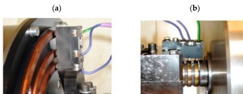
Figure 3. Slip rings and brushes: (a)—the driving part, (b)—the driven part.
