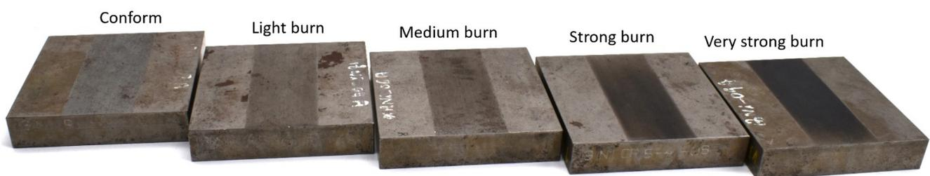
**Figure 2.** Illustration for the five grinding burn levels.
