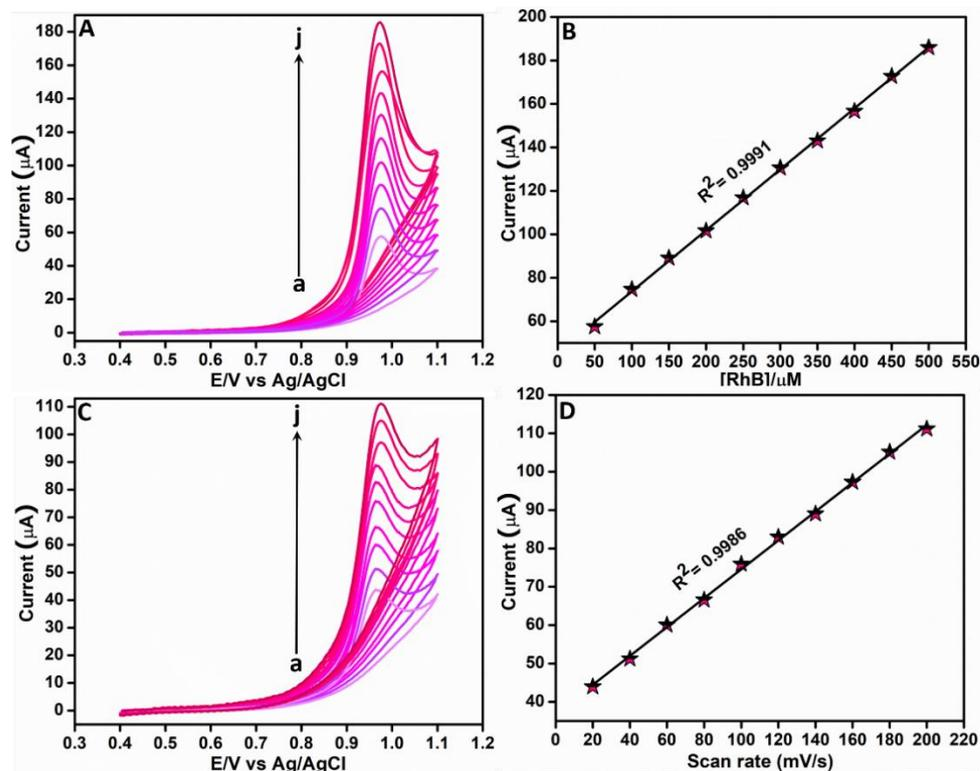
**Figure 6.** (A) Voltammetric curves of Ag-3/ZnO/SPCE under different additions of RhB from 50  $\mu\text{M}$  to 500  $\mu\text{M}$  to 0.05 M PBS (pH 7) at 0.1 V/s and (B) Corresponding linear plot. (C) Voltammetric curves of Ag-3/ZnO/SPCE under different scan rates from 0.02–0.2 V/s and (D) corresponding linear plot.
