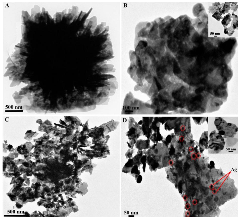
**Figure 2.** TEM images of 3D, hierarchical, nanosheet-based, flower-like ZnO (A,B) and Ag-3/ZnO (C,D). The red dot circle indicates Ag nanoparticles.
