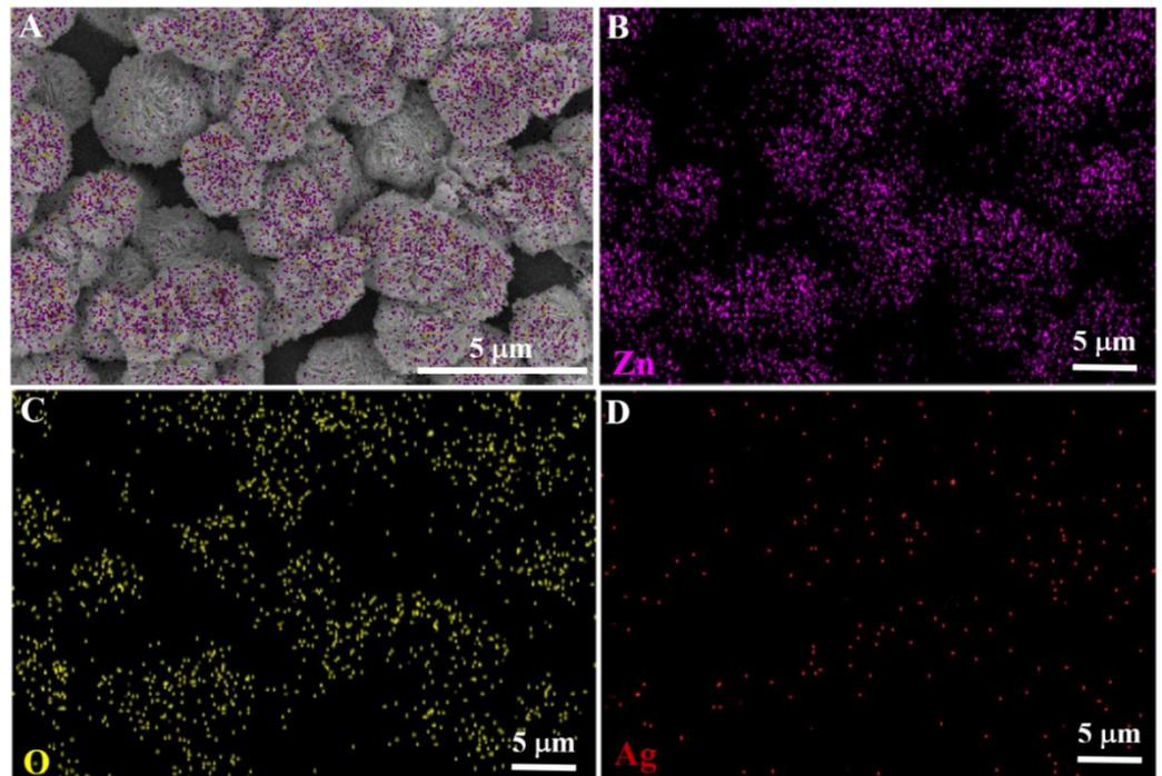
**Figure 3.** SEM of Ag-3/ZnO (A); corresponding elemental mapping of zinc (B), oxygen (C), and silver (D).
