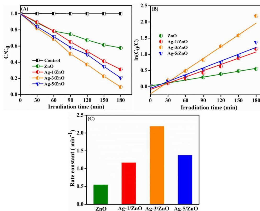
**Figure 9.** Photodegradation of RhB (A), corresponding pseudo-first-order kinetic plots (B), and rate constant plot (C) of ZnO and Ag/ZnO.
