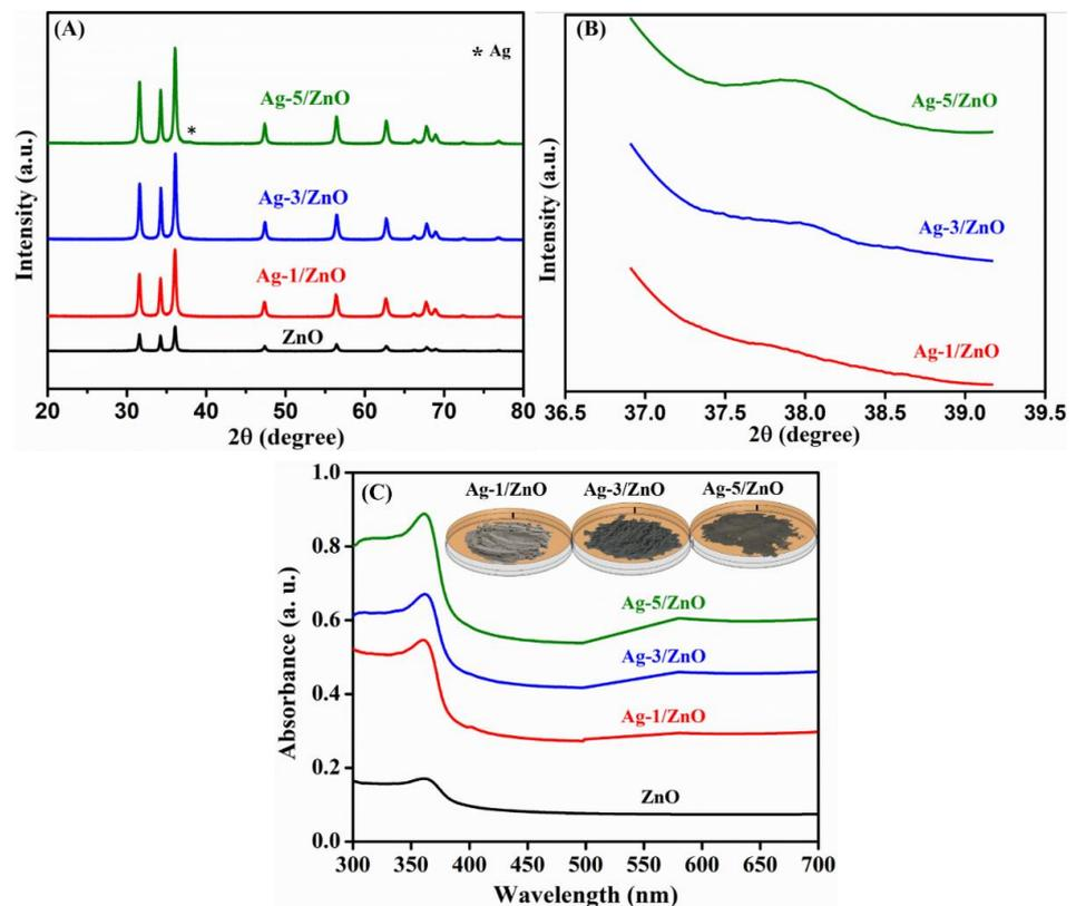
**Figure 4.** The XRD pattern: as-prepared samples (A) and UV-vis absorption spectra (B,C) of pure ZnO, Ag-1/ZnO, Ag-3/ZnO, and Ag-5/ZnO.
