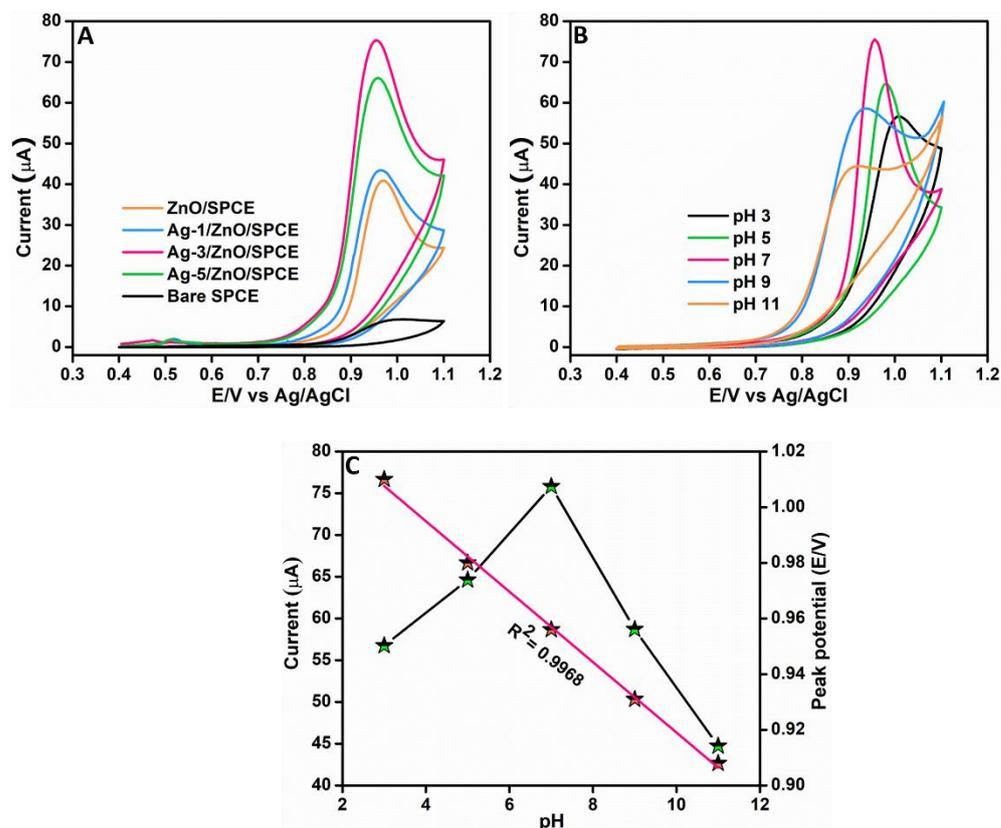
**Figure 5.** Voltammetric curves of different modified electrodes in 0.05 M PBS (pH 7.0) in presence of 100  $\mu$ M RhB at 0.1 V/s (A). Voltammetric curves of Ag-3/ZnO/SPCE at different pH from pH 3 to pH 11 in presence of 100  $\mu$ M RhB at 0.1 V/s (B). The pH against peak current and potential (C).
