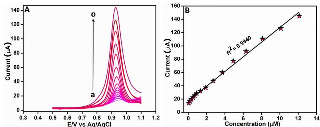
**Figure 7.** (A) DPV curves of Ag-3/ZnO/SPCE under different RhB concentrations in 0.05 M PBS (pH 7). (B) Linear plot of peak currents vs. RhB concentrations.
