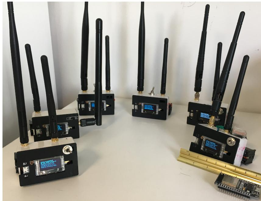
**Figure 9.** Several nodes were built to take part in the WSN field experiments.
