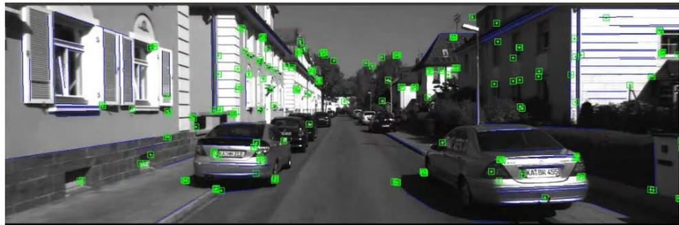
**Figure 1.** The results of point and line features on the KITTI dataset sequence 00. The green boxes represent the point features extracted from the image, and the blue lines are the extracted line features.
