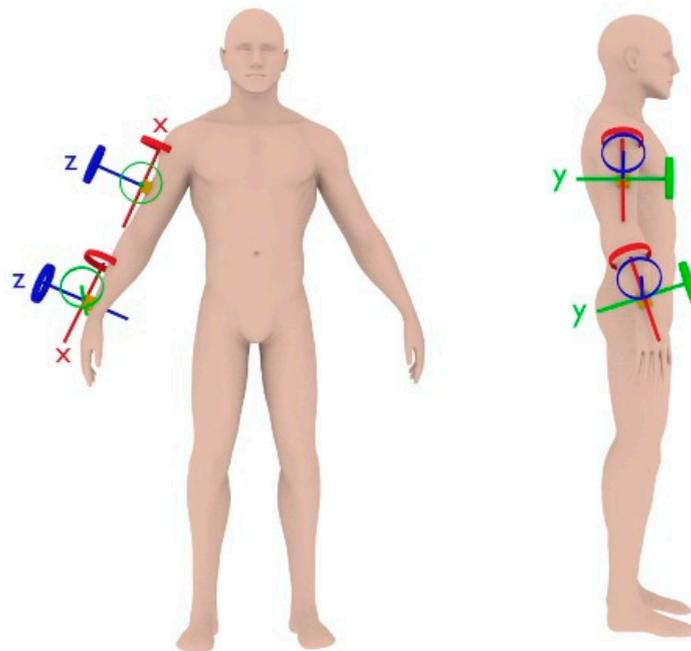
**Figure 1.** IMUs location and relevant coordinate systems in upright standing can be appreciated: Z-axis, anteroposterior; Y-axis, mediolateral; X-axis, vertically aligned with the direction of the gravitational field vector.
