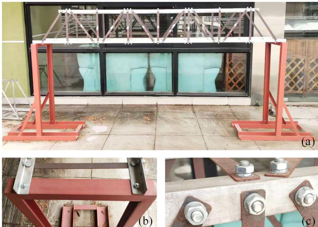
**Figure 3.** The bridge model with 60 flat steel bars. (a) Model layout; (b) boundary condition; (c) connection type.
