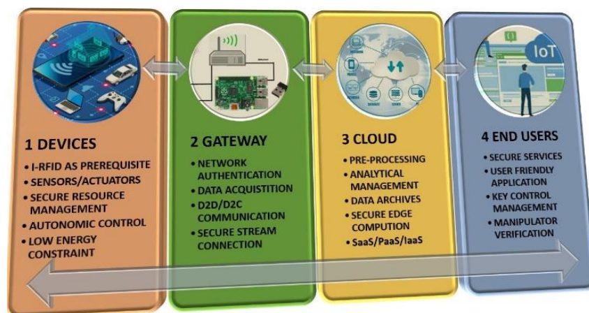
Figure 1. Internet of things (IoT) four-tier architecture for smart X environments. Each tier is linked with each other through internet gateway access. Under this scenario, end users can easily manage and control the devices tier.
