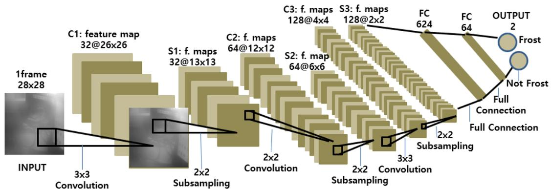
**Figure 4.** Structure of the convolutional neural network (CNN) used for frost detection.
