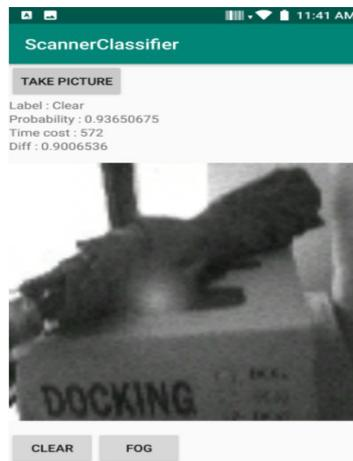
**Figure 3.** Data collection app: It takes a picture, resizes it, and collects the human-provided label to be associated with it.
