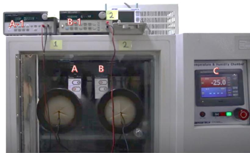
**Figure 13.** Cold-chamber experiment (A: Terminal with existing method; B: Terminal with edge AI method; A-1 and B-1: DC power supplies for measuring the current at Terminal A and B, respectively; C: Cold-chamber controller maintaining  $-25\text{ }^{\circ}\text{C}$ ).
