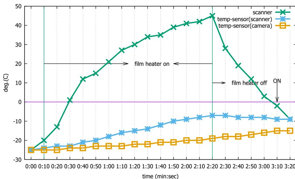
**Figure 9.** Temperature changes on two sensors when the industrial mobile terminal turns on and then turns off the film heater; without edge artificial intelligence (AI) logic.
