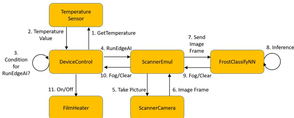
Figure 7. System state diagram.
