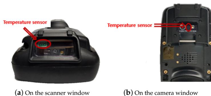
Figure 8. Temperature sensors on the test platform (UL20f).
