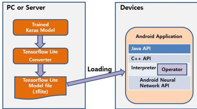
Figure 6. Loading the trained model to our industrial mobile terminal.
