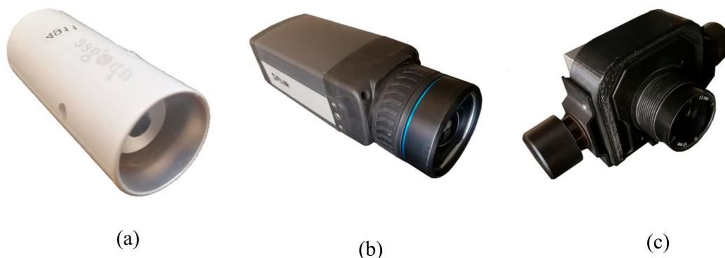
**Figure 1.** Instruments calibrated during this study (a) Apogee SI-111 infrared radiometer, (b) FLIR A655sc uncooled radiometric thermal camera, (c) TeAx 640 miniature uncooled radiometric thermal camera for unmanned aerial vehicle (UAV) applications.
