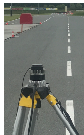
Figure 17. Schematic illustration of measurements setup including the Ouster OS-1-64 [24] and three Lambertian targets from SphereOptics [27] with defined reflectance values R_\lambda(L) at 10%, 50%, and 95%.
