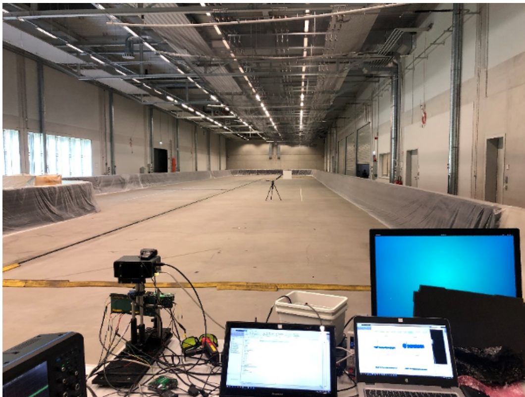
Figure 15. Lidar measurement setup in the indoor test-facility Carissma. The Infineon lidar prototype is pointed towards a Lambertian target that is mounted on a tripod and placed at different distances.
