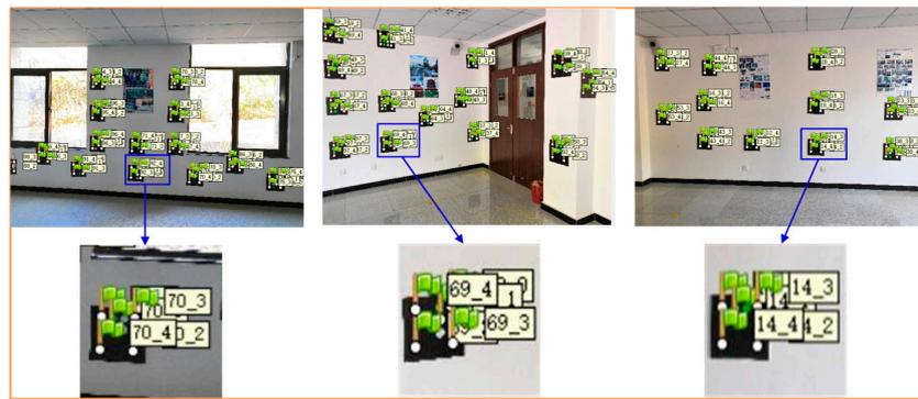
Figure 8. Identified color encoded targets.
