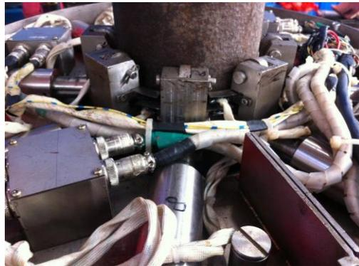
**Figure 14.** The lift-off-tolerant MFL probing system.
