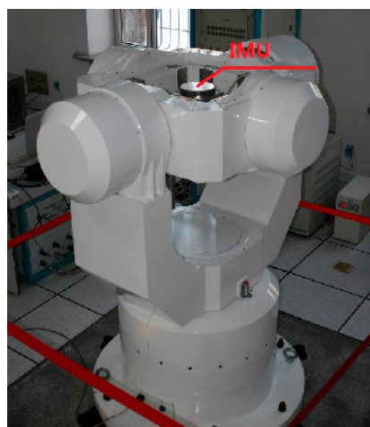
Figure 7. Three-axis turntable for experiments.
