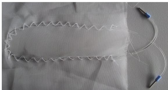
The sensing textiles were sewed on the inside of a custom developed chest strap which consisted of polyester textile, rubber straps and a buckle. Afterwards the strap was placed on a test subject (28 year old, male, 182 cm, 72 kg) as shown in Figure 2.
