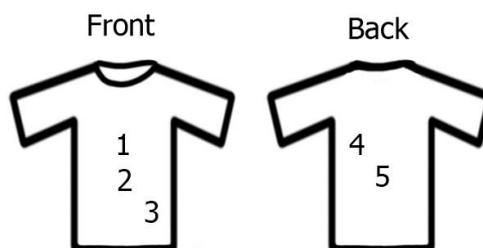
Figure 8 compares the measurements from the above-mentioned breathing types. Figure 8a presents the measurements while the subject was performing diaphragmatic breathing, the best signal change was obtained when the sensor setup was placed above the navel (position 2) ( $0.027 \pm 0.003$  V). Signal artefacts were not observed. As discussed in the introduction, the girth around the abdominal
