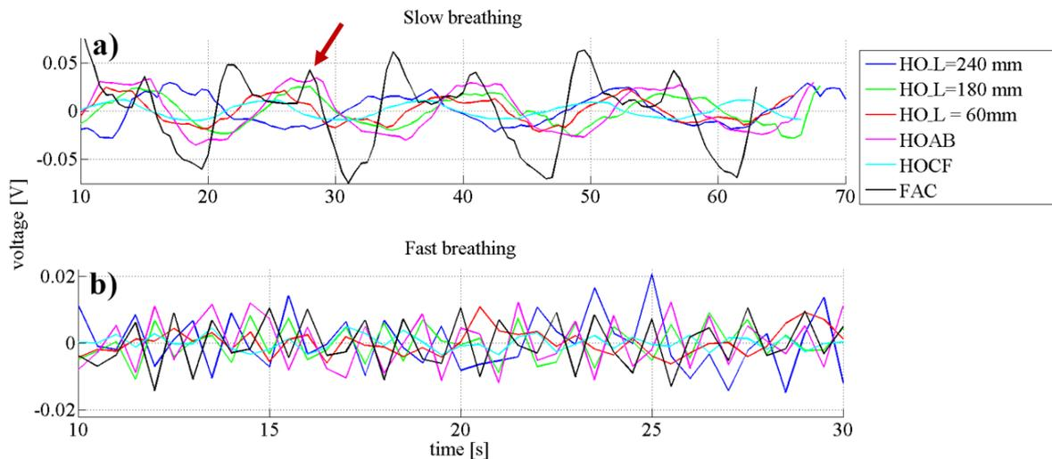
In Figure 6b the graphs of the fast breathing scenario are presented. The plotting from the  $HOL = 60$  mm was nearly flat and no peaks that would correspond to the respiratory rate were detected. All the other samples had similar amplitude changes in the range of  $0.010 \pm 0.03$  V.
