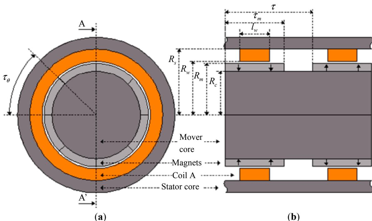
Two ring-shaped coils, each one with 64 turns, are made of standard 12 AWG enameled copper wire. Each coil is positioned in front of the corresponding pole face of the permanent magnet, producing force in the axial direction when electric current is properly applied to them. These coils are connected in series in a way that the current is established in the coils in opposite directions with respect to each other. The actuator has only one phase, making it simple to control its position and
