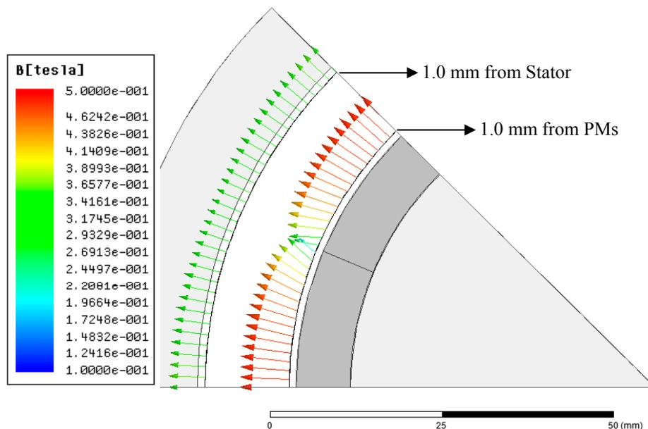
Figure 10 also shows that the component is higher close to the permanent magnets and tends to zero near the stator core. This effect is due to the fact that the flux lines follow the path of least magnetic reactance and for this reason they align in the radial direction in the air gap. In this figure it can be observed that the mean value of the tangential component is zero.
