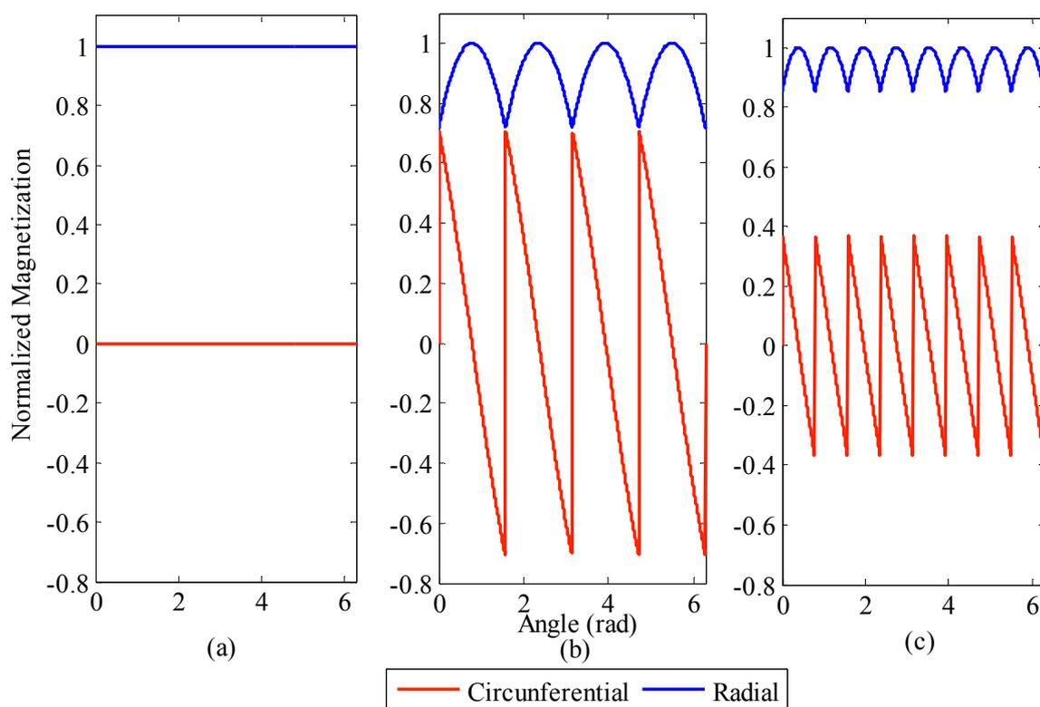
Figure 4 indicates that the mean value of the circumferential component of the magnetization is zero. Actually, it is so regardless of the number of segments. It can also be understood that the amplitude of the circumferential component will be greater the smaller the number of segments with parallel magnetization.
