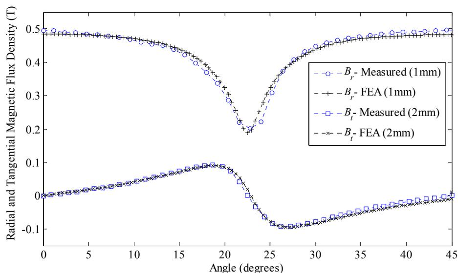
Results of normal and tangential components of flux density measured with a model FH54—Magnet Physik® Teslameter are shown in Figure 18. The normal component presents a peak value of 0.49 T and the minimum value is 0.2 T, while the mean value is 0.43 T, which represents a reduction of 12.2%
