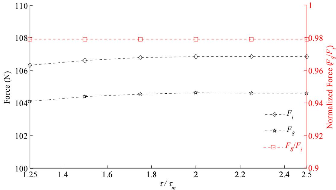
Although there is a variation in the resultant force with the variation of  $\tau/\tau_m$ , the normalized force,  $\tilde{F}_8$ , is nearly constant, which also suggests that the variation is not affected by the magnetization pattern. In a similar way as the analysis of the armature reaction, the ratio  $\tau/\tau_m$  has influence in the flux density distribution on the axial direction, so that in the  $r\theta$  plane it is affected equivalently for both magnetization patterns.
