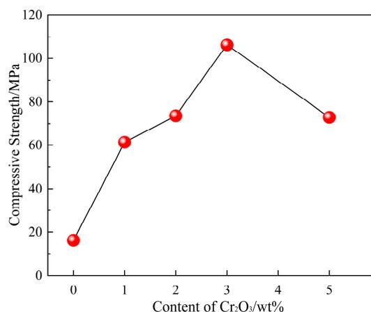
**Figure 9.** Effect of  $\text{Cr}_2\text{O}_3$  content on the compressive strength of the sinter.
