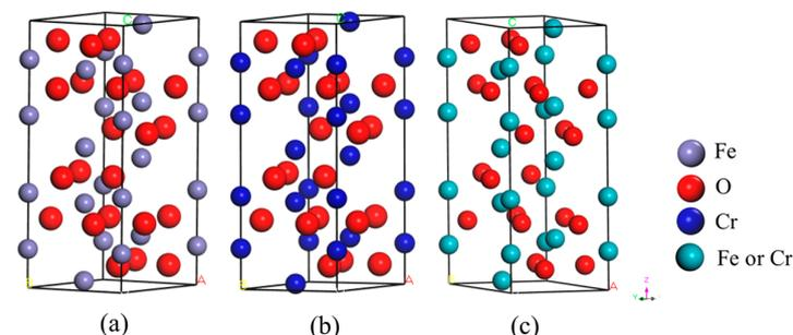
Figure 2. Crystal structures of  $\text{Fe}_2\text{O}_3$ ,  $\text{Cr}_2\text{O}_3$  and  $(\text{Fe}_{1-x}\text{Cr}_x)_2\text{O}_3$ : (a)  $\text{Fe}_2\text{O}_3$ ; (b)  $\text{Cr}_2\text{O}_3$ ; (c)  $(\text{Fe}_{1-x}\text{Cr}_x)_2\text{O}_3$ .
