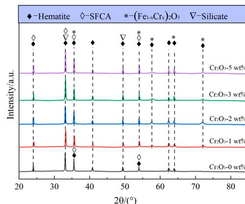
Figure 1. XRD patterns of samples with different  $\text{Cr}_2\text{O}_3$  contents.
