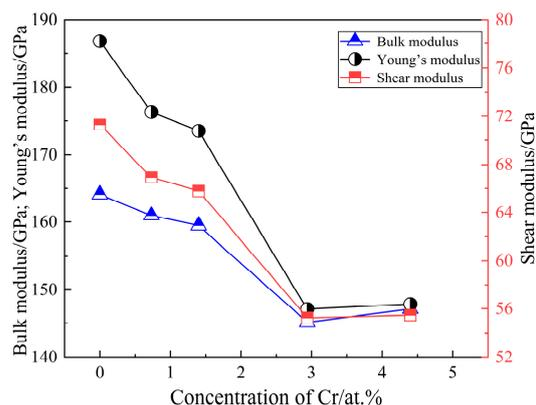
**Figure 5.** Bulk modulus, shear modulus, and Young's modulus for SFCA crystals with different doped Cr concentrations.
