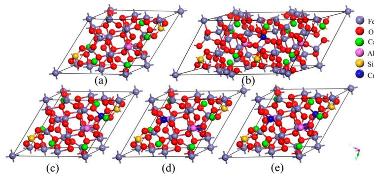
**Figure 11.** SFCA cells with different Cr doping amounts: (a) 0 at.%; (b) 0.73 at.%; (c) 1.40 at.%; (d) 2.94 at.%; (e) 4.40 at.%.
