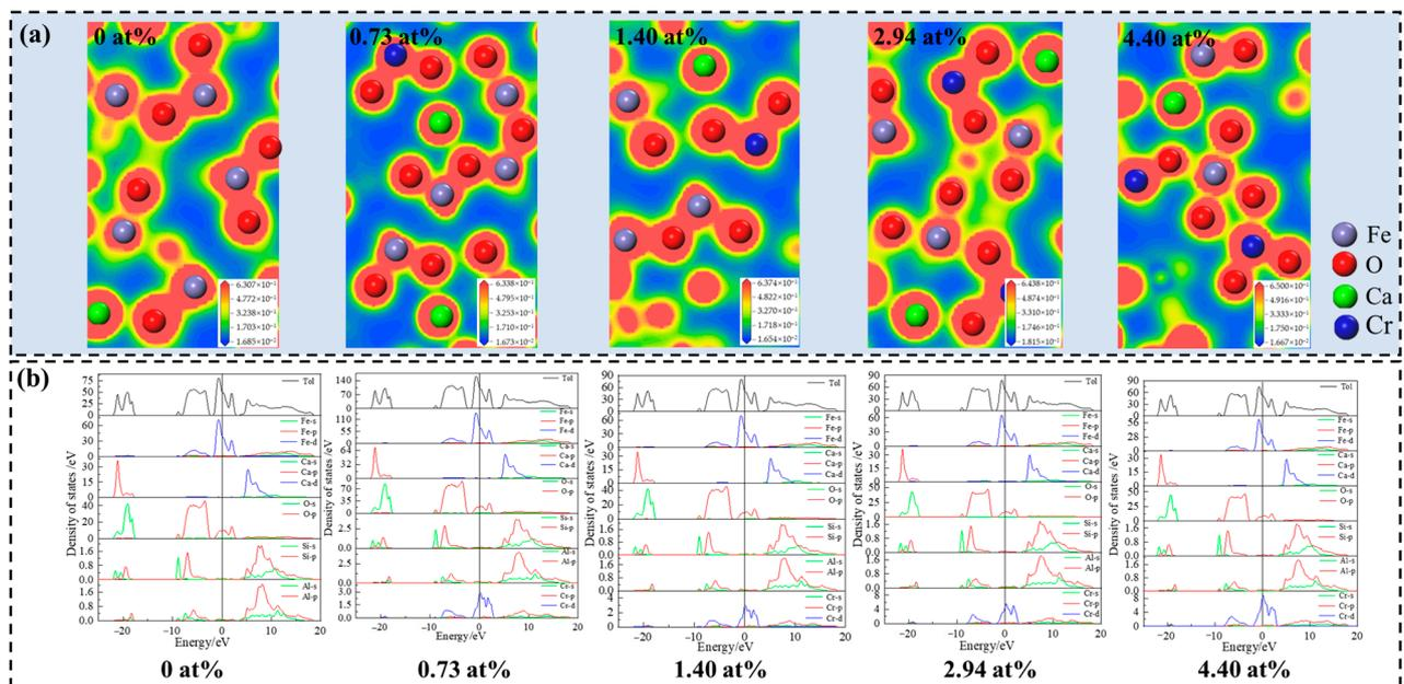
**Figure 6.** (a) The electron density distribution of SFCA crystals doped with different doped Cr concentrations; (b) the density of states of SFCA crystals doped with different doped Cr concentrations.
