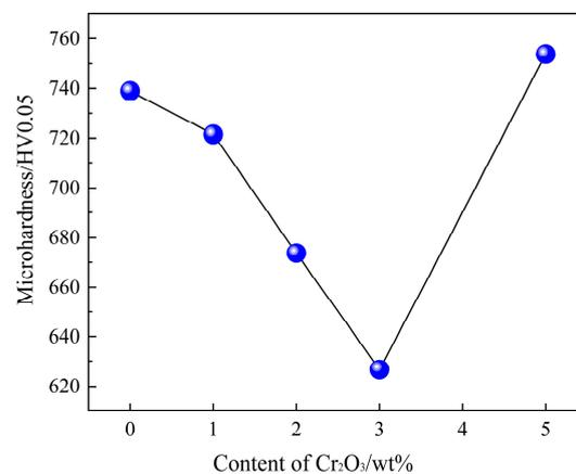
**Figure 8.** Effect of  $\text{Cr}_2\text{O}_3$  content on microhardness of SFCA.
