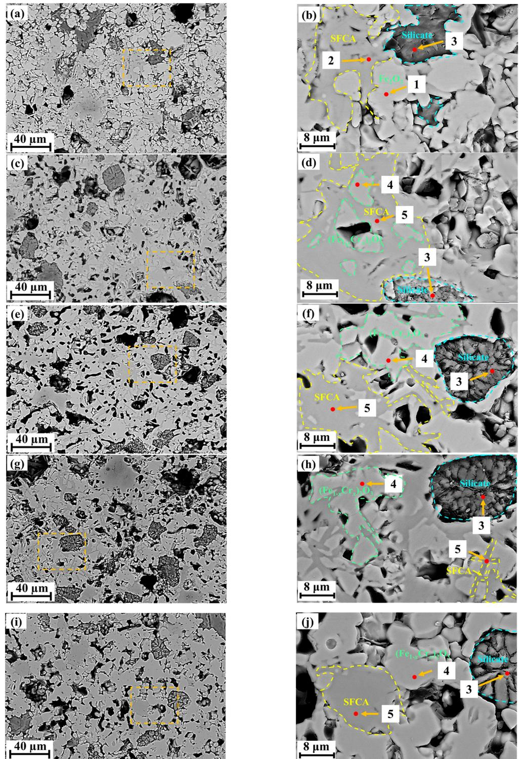
**Figure 3.** SEM results of samples with different  $\text{Cr}_2\text{O}_3$  content. (a,b): 0 wt%  $\text{Cr}_2\text{O}_3$ ; (c,d): 1 wt%  $\text{Cr}_2\text{O}_3$ ; (e,f): 2 wt%  $\text{Cr}_2\text{O}_3$ ; (g,h): 3 wt%  $\text{Cr}_2\text{O}_3$ ; (i,j): 5 wt%  $\text{Cr}_2\text{O}_3$ ; (b,d,f,h,j) are enlarged images of the enclosed areas of (a,c,e,g,i), respectively.
