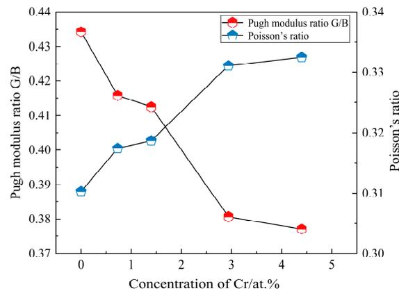
**Figure 7.** G/B values and Poisson's ratio for SFCA crystals doping with different Cr concentrations.
