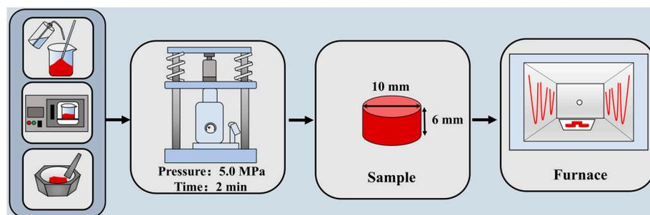
**Figure 10.** Process schematic of sample preparation and sintering.
