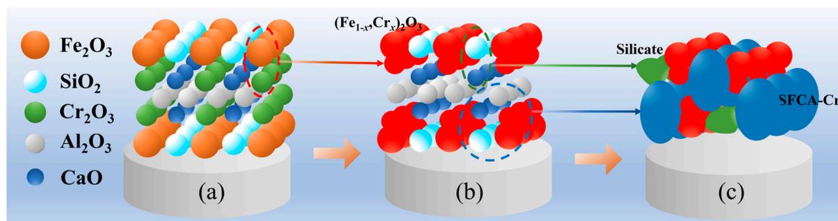
**Figure 4.** Formation mechanism of SFCA with Cr.
