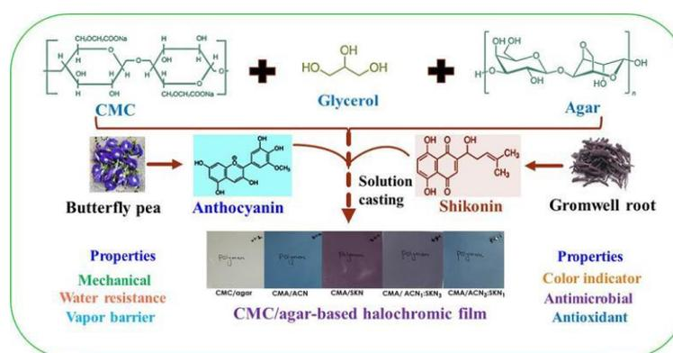
**Figure 2.** Schematic diagram of the fabrication of carboxymethyl cellulose (CMC)/agar-based functional color-changing membranes [26].
