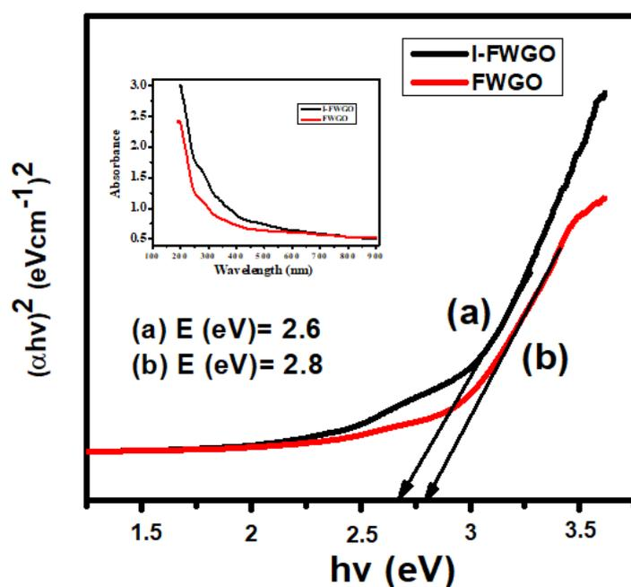
Figure 4. Bandgap of (a) I-FeWO<sub>4</sub>/GO and (b) FeWO<sub>4</sub>/GO.
