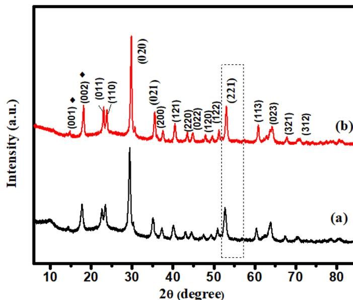
Figure 2. XRD spectra: (a) FeWO<sub>4</sub>/GO; (b) I-FeWO<sub>4</sub>/GO.
