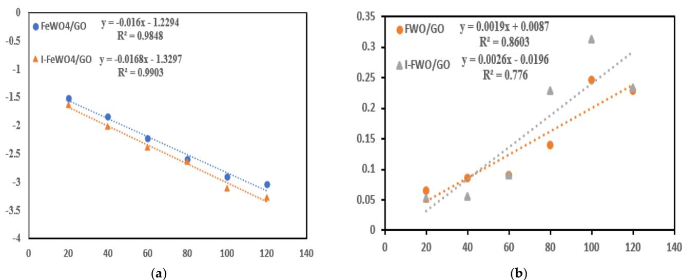
**Figure 7.** Reaction kinetics: (a) first-order kinetics; (b) second-order kinetics of FeWO<sub>4</sub>/GO and I-FeWO<sub>4</sub>/GO.
