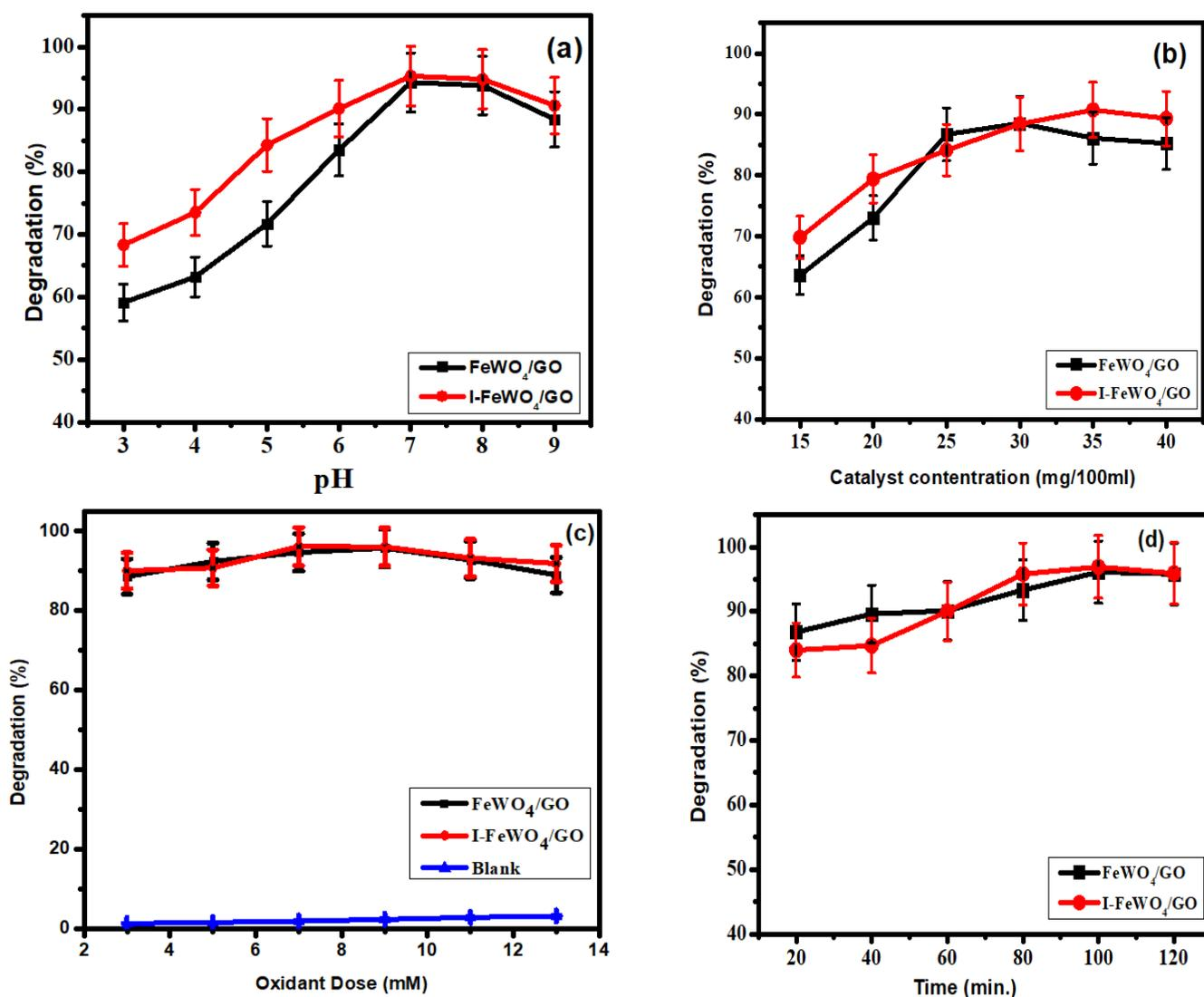
Figure 5. Optimized parameters: (a) pH; (b) catalyst load; (c) oxidant dose (H<sub>2</sub>O<sub>2</sub>); (d) time.
