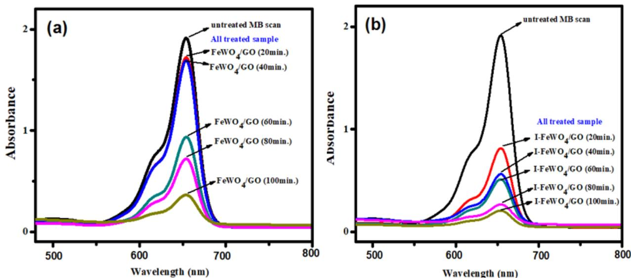
**Figure 6.** MB UV–Vis spectral changes during degradation over time using (a) FeWO<sub>4</sub>/GO and (b) I-FeWO<sub>4</sub>/GO.
