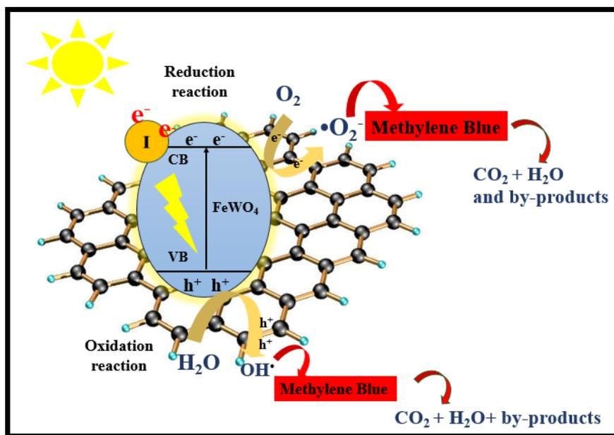
Figure 10. The proposed mechanism for the catalytic degradation of MB using I-FeWO<sub>4</sub>/GO.
