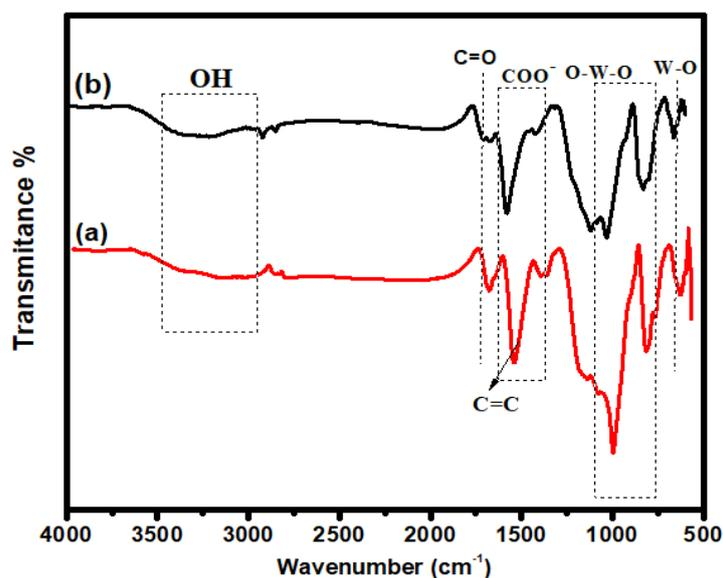
Figure 1. FTIR spectra: (a) FeWO<sub>4</sub>/GO; (b) I-FeWO<sub>4</sub>/GO.
