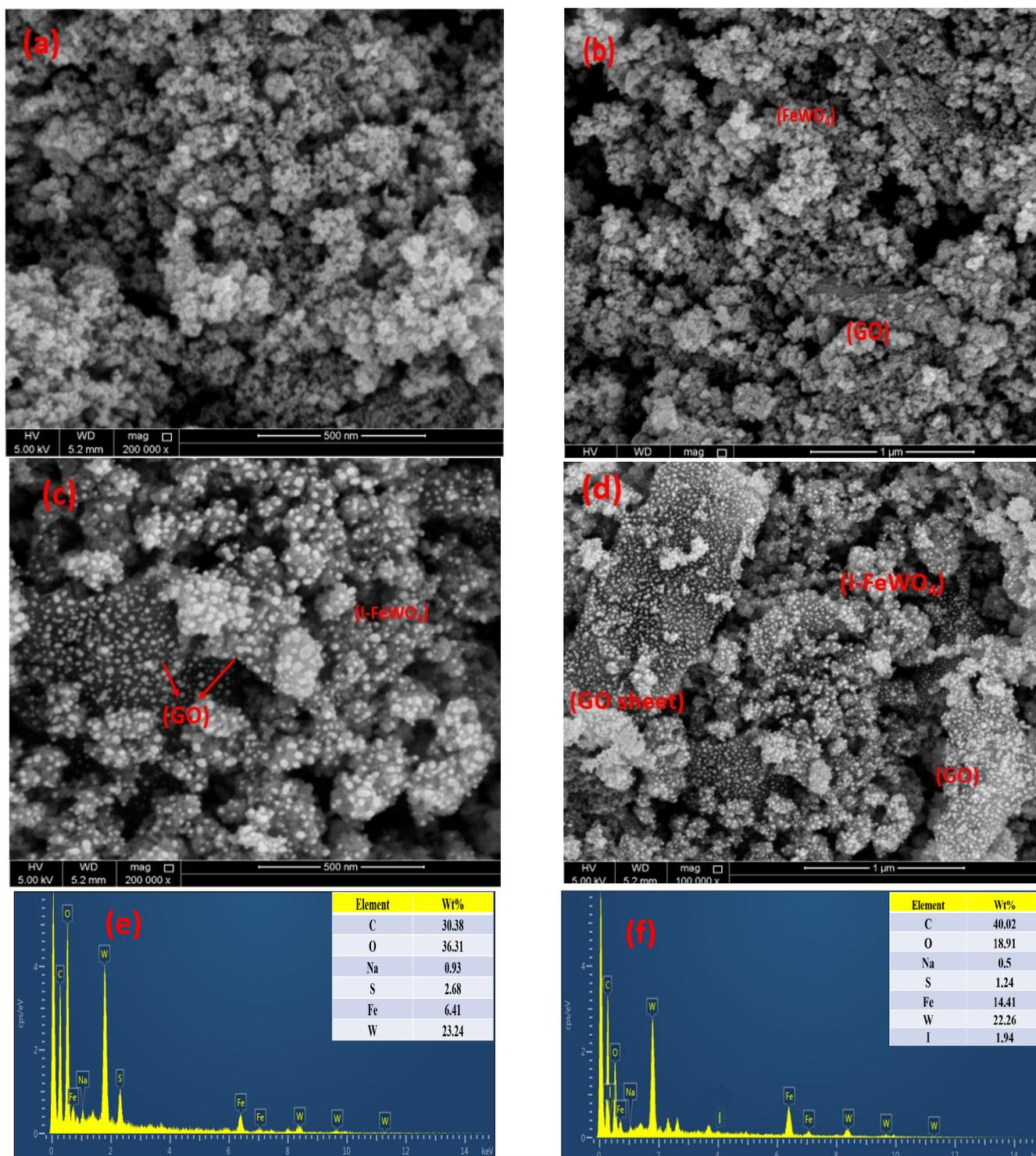
**Figure 3.** SEM images of  $\text{FeWO}_4\text{-GO}$  (a,b) and  $\text{I-FeWO}_4\text{/GO}$  (c,d) and EDX images of (e)  $\text{FeWO}_4\text{-GO}$  and (f)  $\text{I-FeWO}_4\text{/GO}$ .
