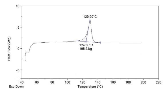
Figure S1. DSC thermogram of polymer material recovered as by-product in EXP1.
