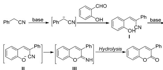
**Scheme 4.** Proposed mechanism of the synthesis of chromenone.
