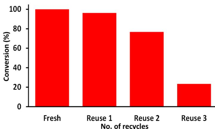
Figure 10. Graphical illustration of conversion product obtained upon catalyst reuse.
