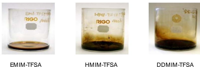
**Figure 10.** Photographs of samples kept at 150 °C.
